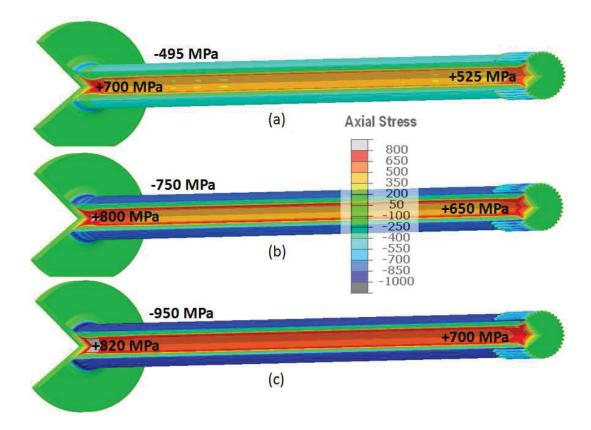
*Figure 9: Axial residual stresses. With heat transfer coefficient of (a) 5K, (b) 12K, and (c) 25K W/(m^2 \cdot C).*
