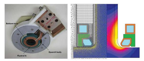
Figure 3: (a) Full assembly of a two-turn axle scan coil with quench body, (b) Fillet area of axle modelled with Flux 2D, mesh elements.
