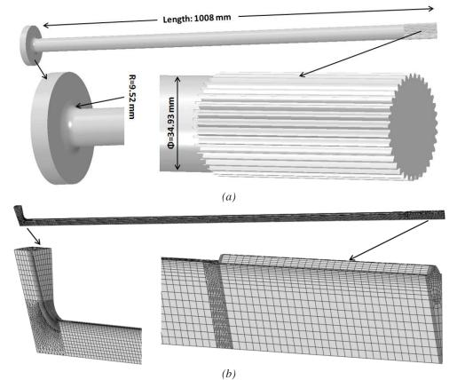
Figure 1: (a) CAD model, and (b) single spline tooth FEA model of the full-float truck axle.
