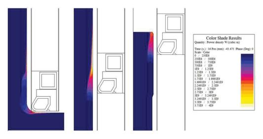
Figure 4: Power density distribution in fillet area at end of dwell (left), shaft (middle), and spline at end of heat (right).
