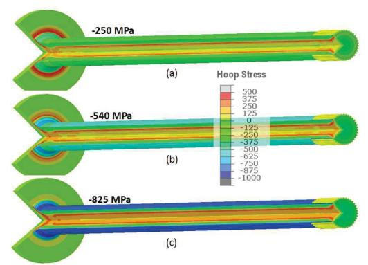
Figure 10: Hoop residual stresses. With heat transfer coefficient of (a) 5K, (b) 12K, and (c)  $25K (W/m^2 \cdot C)$ .
