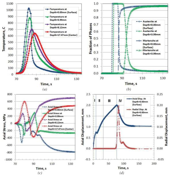
Figure 13: Relationship between temperature, phase transformation, stress, and displacement with heat transfer coefficient of  $12K W/(m^2 \cdot C)$  as boundary condition.
