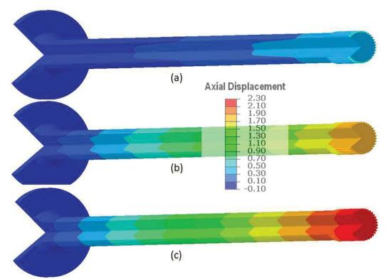
Figure 11: Axial distortion. With heat transfer coefficient of (a) 5K, (b) 12K, and (c)  $25K (W/m^2 \cdot C)$ .
