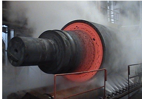
Differential hardening process applied to roll body provides a hardened, compressive surface layer
