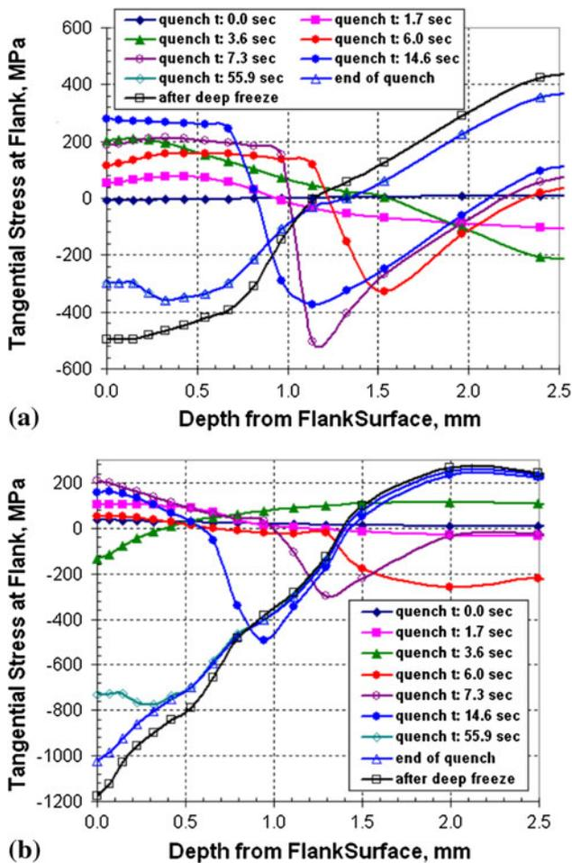
Fig. 6 Stress evolution due to thermal gradient and phase transformation (a) gear flank and (b) root fillet
