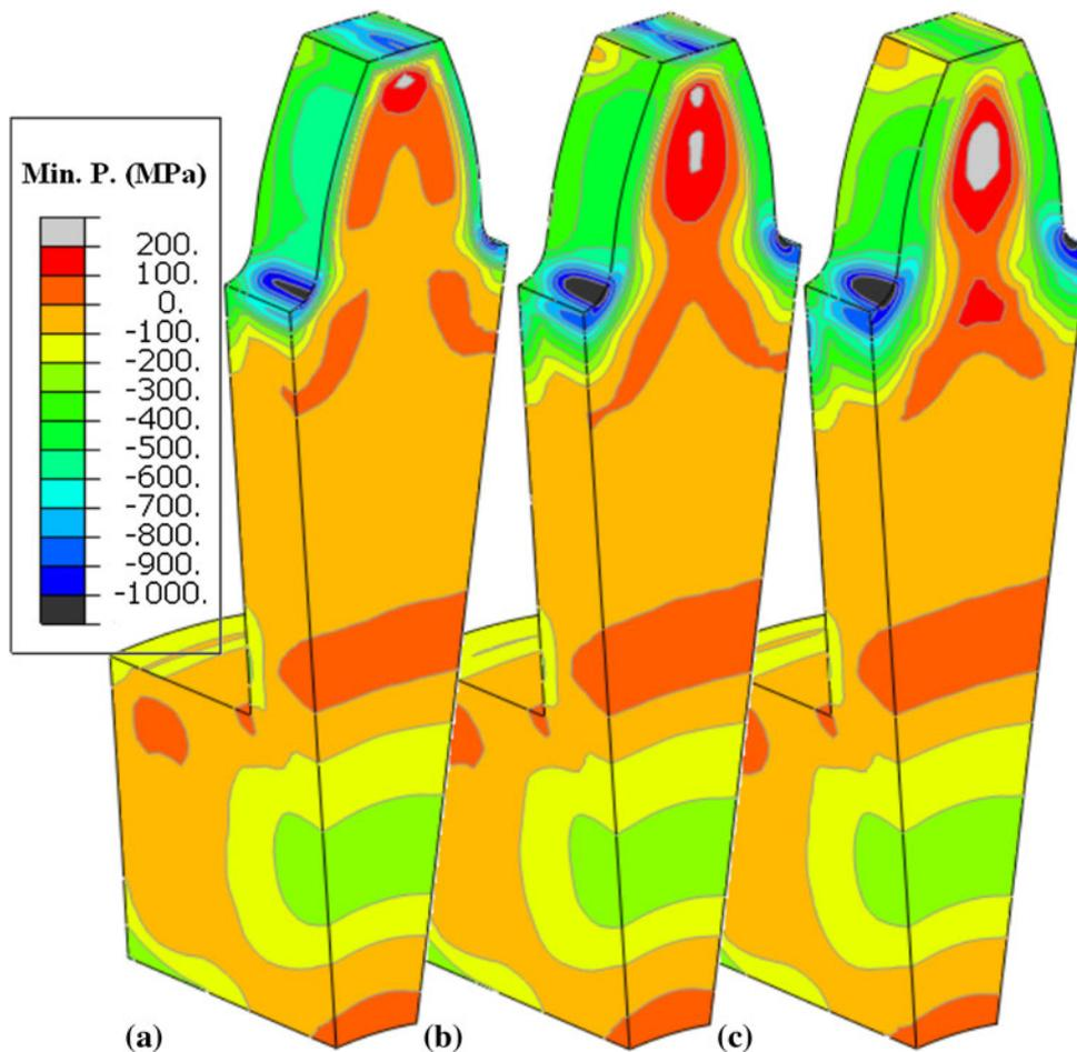
**Fig. 5** Cut view of residual stress distributions for three carbon cases. (a) 0.5 mm, (b) 1.0 mm, and (c) 1.5 mm
