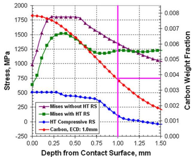
**Fig. 11** Relation between contact stresses and design of carbon case depth
