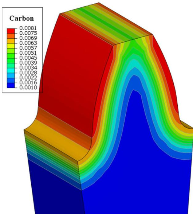
Fig. 2 Carbon distribution contour with case depth of 1.5 mm
