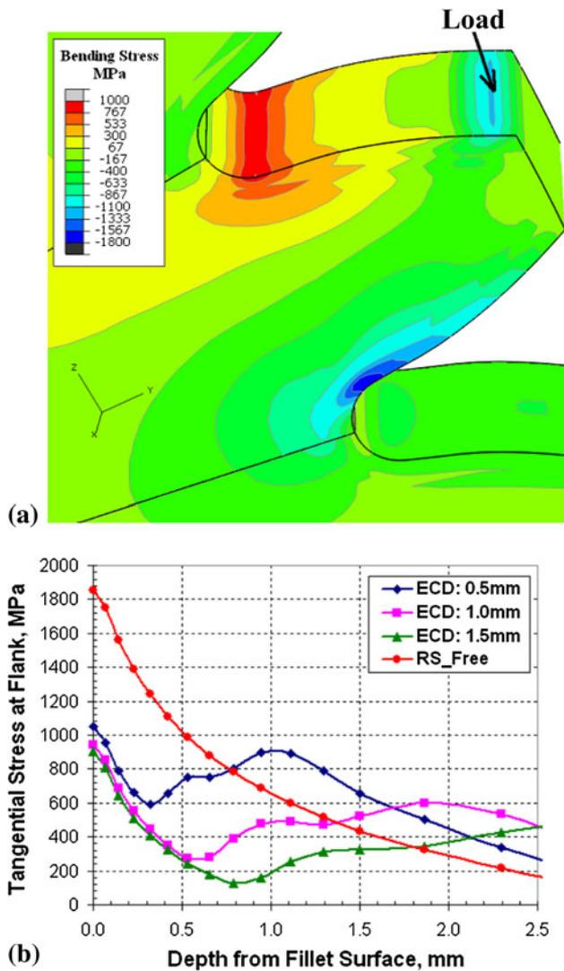
**Fig. 9** Single-tooth bending stress distribution. (a) Contour plot for 1.0 mm carbon case depth and (b) stress distribution in terms of depth
