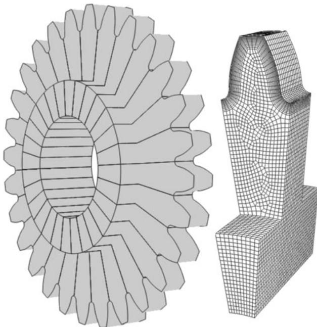
**Fig. 1** Gear geometry and finite element mesh of single tooth model
