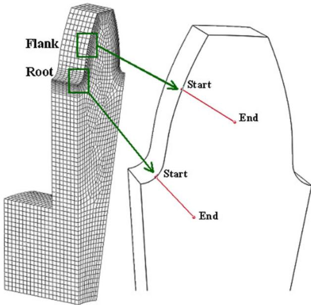
Fig. 3 Cross section and two straight lines selected for modeling result analysis
