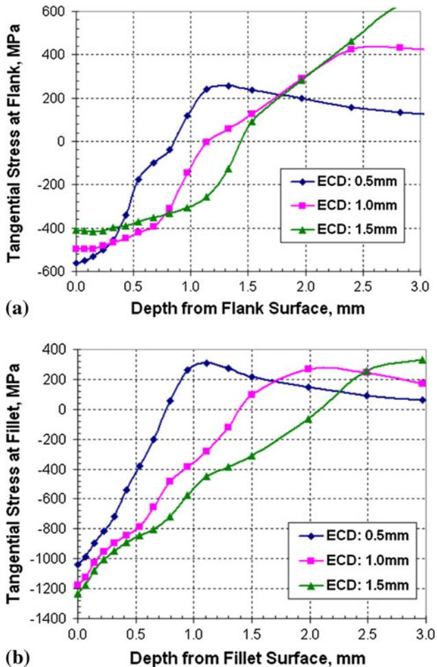
Fig. 8 Predicted residual stresses in terms of depth from three carburization case depths at (a) root fillet and (b) gear flank regions
