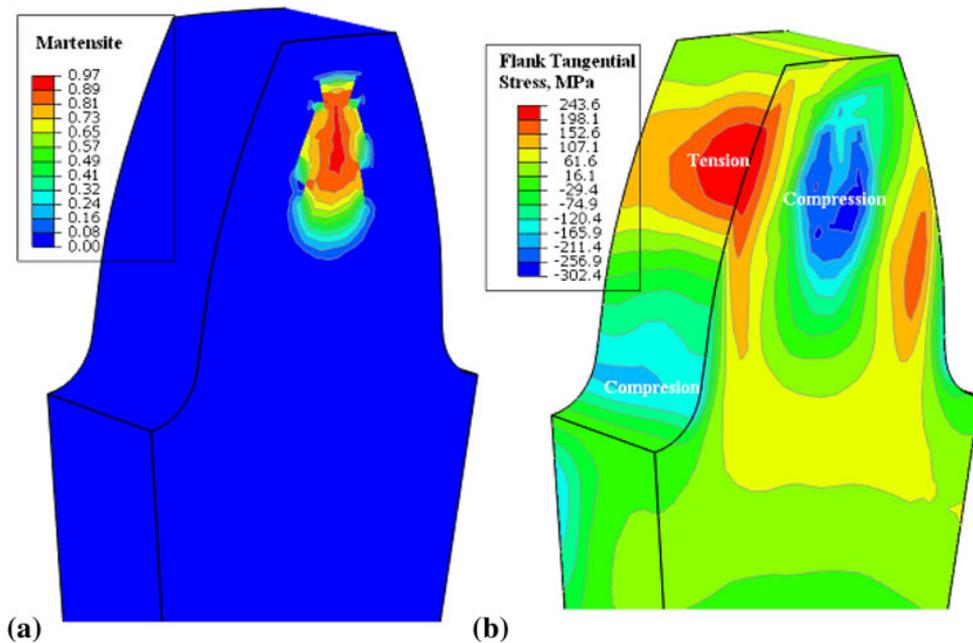
Fig. 7 Cut view of (a) martensite distribution and (b) stress distribution, at 3.6 s during quench using the 1.0 mm effective case depth study
