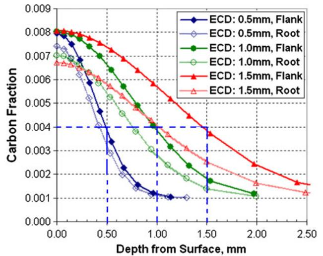
Fig. 4 Carbon distributions in terms of depth and increased geometry effect with case depth
