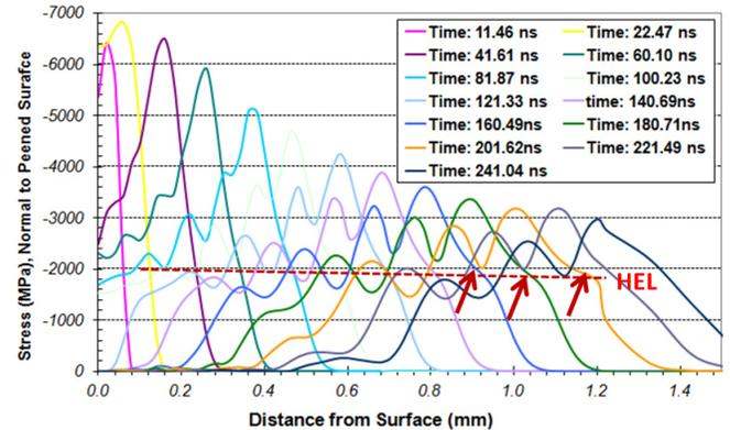
**FIGURE 7 – SHOCK WAVE PROPAGATION THROUGH THE MATERIAL FROM SINGLE SHOT.**
