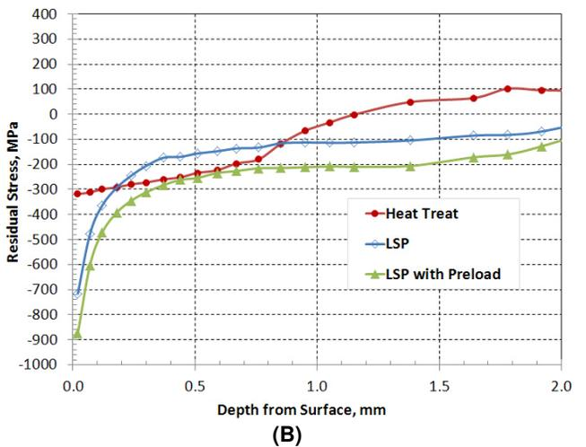
**FIGURE 11 – COMPARISON OF PREDICTED RESIDUAL STRESSES. (A) THROUGH THE SAMPLE THICKNESS, AND (B) ZOOMED IN PLOT CLOSING TO SURFACE.**
