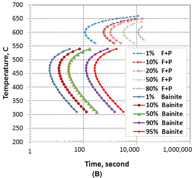
**FIGURE 3 - (A) DILATOMETRY STRAIN CURVE DURING CONTINUOUS COOLING, AND (B) TTT DIAGRAMS OF AISI 9310 GENERATED FROM DANTE DATABASE.**
