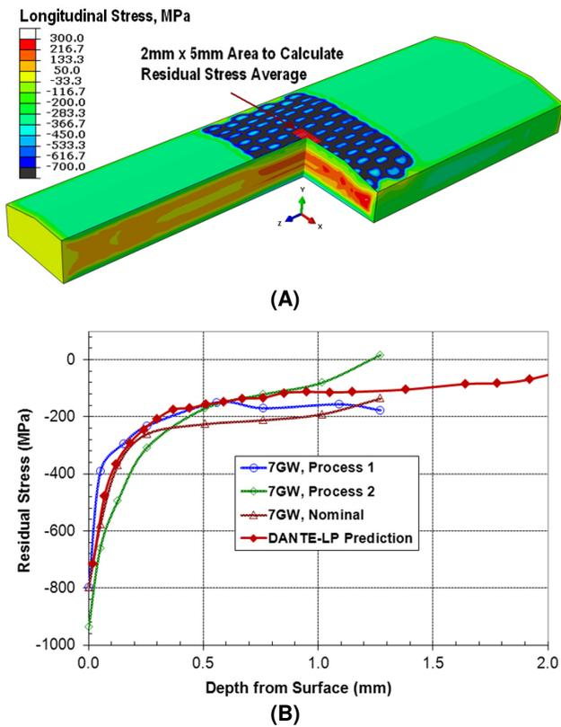
**FIGURE 8 - RESIDUAL STRESSES IN THE LONGITUDINAL DIRECTION AFTER LASER PEENING. (A) CONTOUR PLOT PREDICTED BY DANTE-LP, AND (B) COMPARISON BETWEEN PREDICTION AND X-RAY DIFFRACTION MEASUREMENTS [15].**
