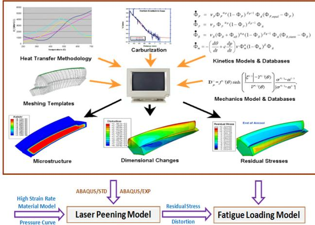
**FIGURE 1 - INTEGRATED COMPUTER MODELING FOR CRABURIZATION, QUENCH HARDENING, LASER PEENING, AND FATIGUE LOADING.**
