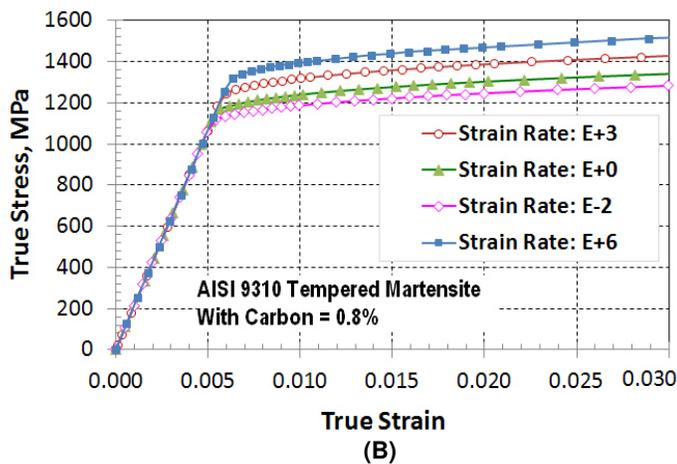
**FIGURE 4 - HIGH STRAIN RATE PLASTIC PROPERTIES OF AISI 9310 (TEMPERED MARTENSITE). (A) 0.1 wt.% CARBON, AND (B) 0.8 wt.% CARBON.**
