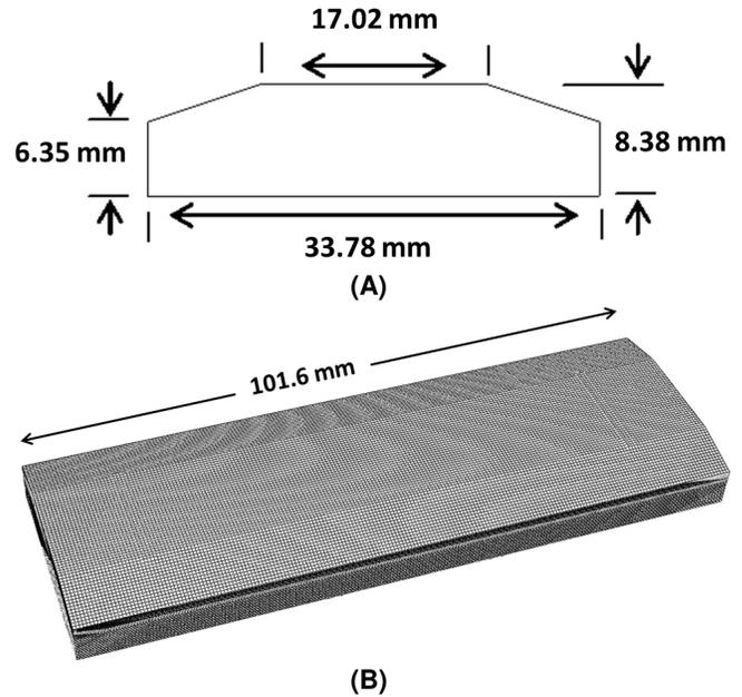
**FIGURE 2 - (A) GEOMETRY, AND (B) FINITE ELEMENT MESH OF THE HERSHEY SAMPLE.**
