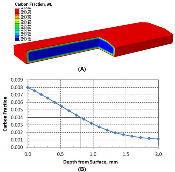
**FIGURE 5 - CARBON DISTRIBUTION. (A) CONTOUR PLOT, AND (B) CURVE PLOT IN TERMS OF DEPTH.**
