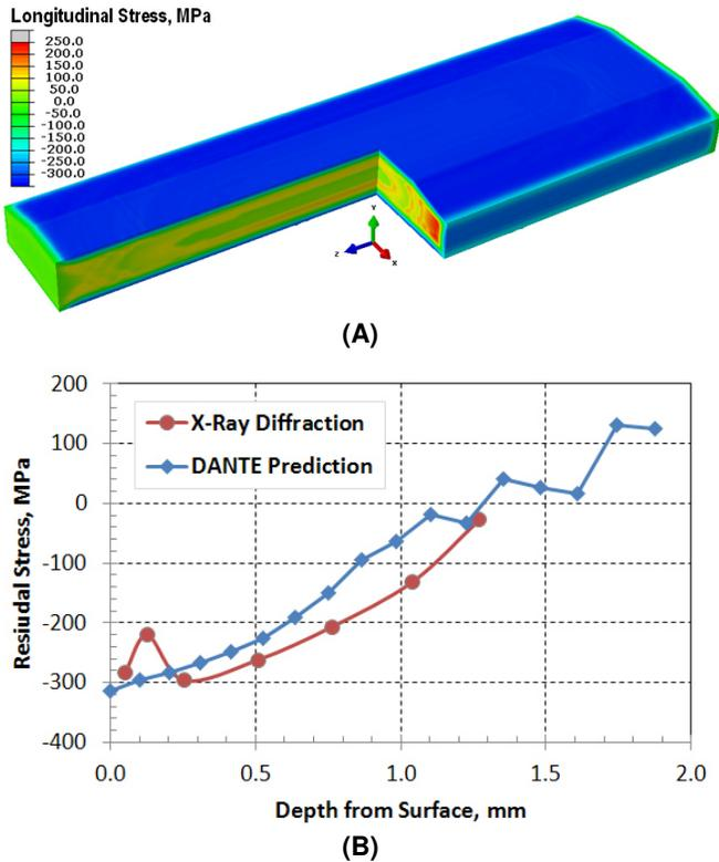
**FIGURE 6 - RESIDUAL STRESSES IN THE LONGITUDINAL DIRECTION AFTER QUENCHING HARDENING. (A) CONTOUR PLOT PREDICTED BY DANTE, AND (B) COMPARISON BETWEEN DANTE PREDICTION AND X-RAY DIFFRACTION MEASUREMENT [15].**
