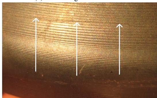
(b) Higher Magnification of Crack.
