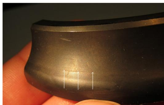
(a) Low Magnification of Crack.
