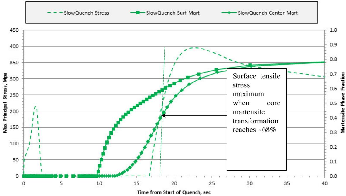
Figure 16 – Stress-Martensite-Time plot for the low heat transfer press quench (Case #2), showing how the delayed core transformation produces the transient tensile stress “spike” on the outer ring surface.
