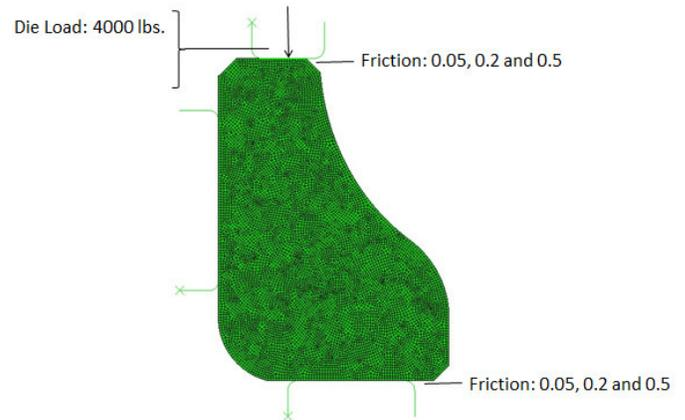
**Figure 6 – Schematic illustrating press quench loading and frictional boundary conditions applied to the 52100 ring heat treatment model.**
