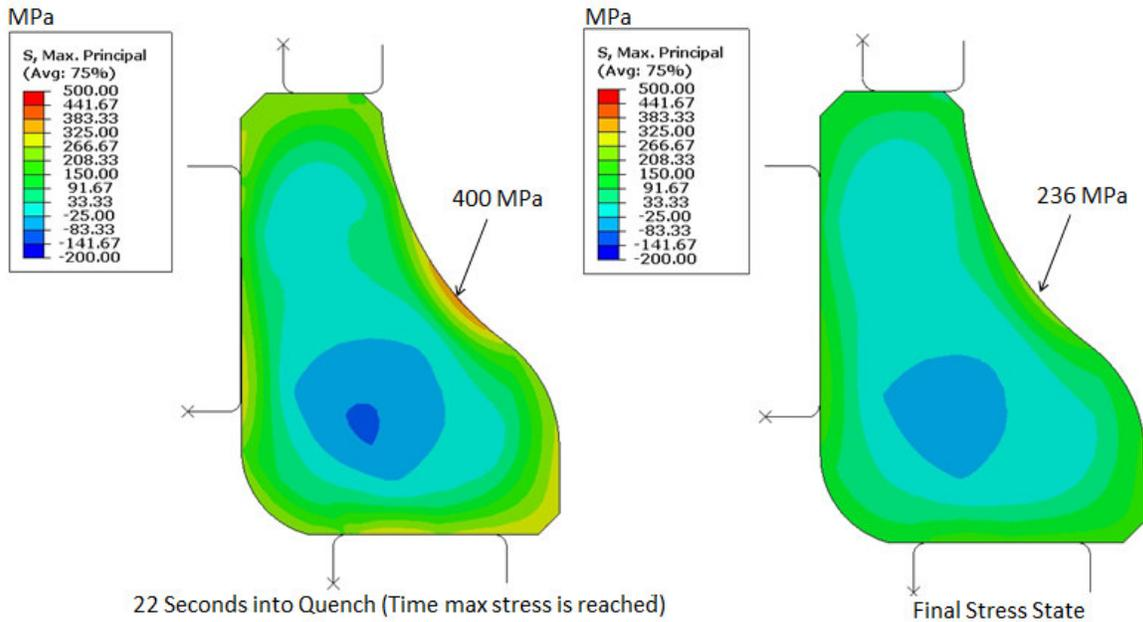
Figure 9 – Maximum principal stress at 22 seconds into press quench and at the end of the press quench, for the low heat transfer quench condition. (Case #2 in Table IV)
