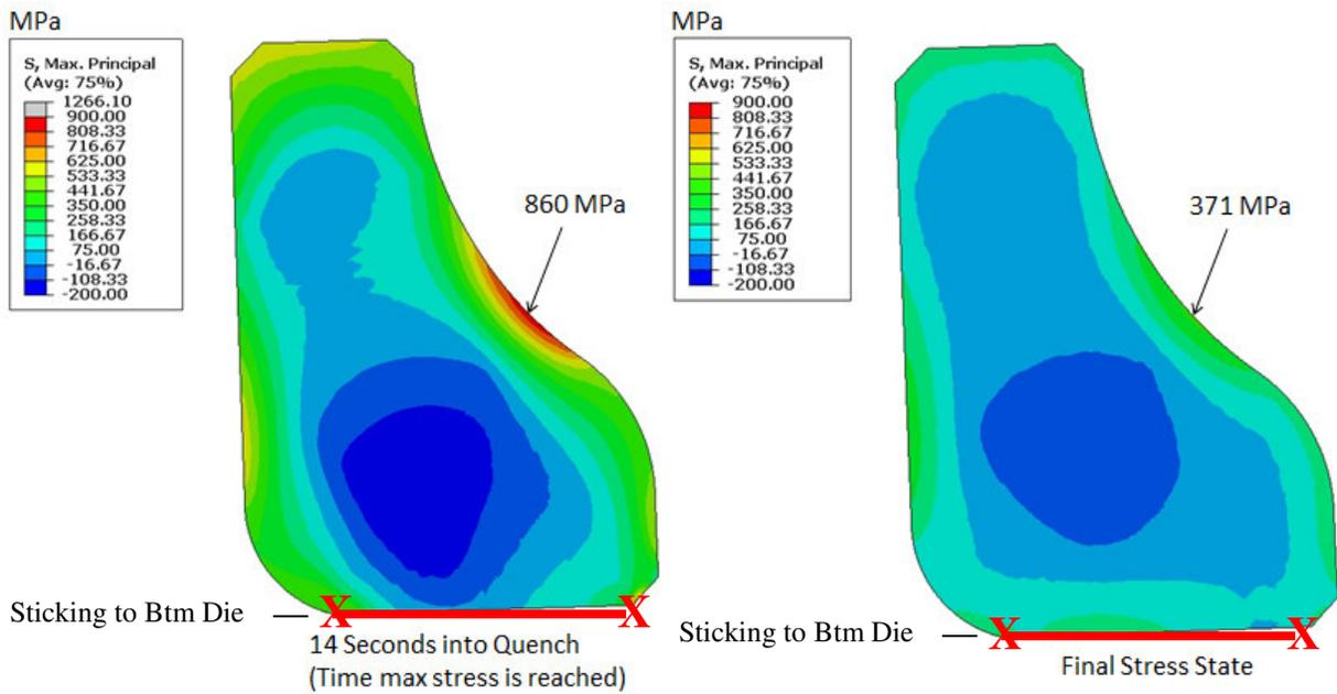
Figure 13 – Maximum principal stress at 14 seconds into press quench, with “Sticking” of the ring bottom surface (radial displacement restriction). Case #8 in Table IV)
