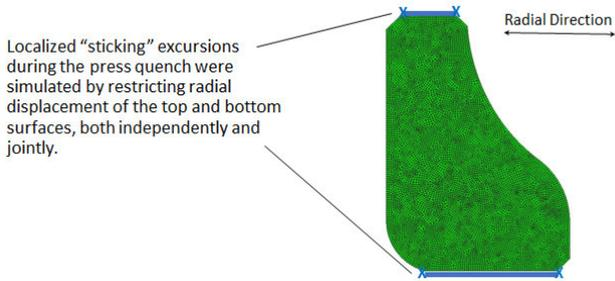
**Figure 7 – Benefit of pulsing the dies was determined by modeling sticking friction during the press quench by restricting radial displacements of the top and bottom surfaces of the ring.**
