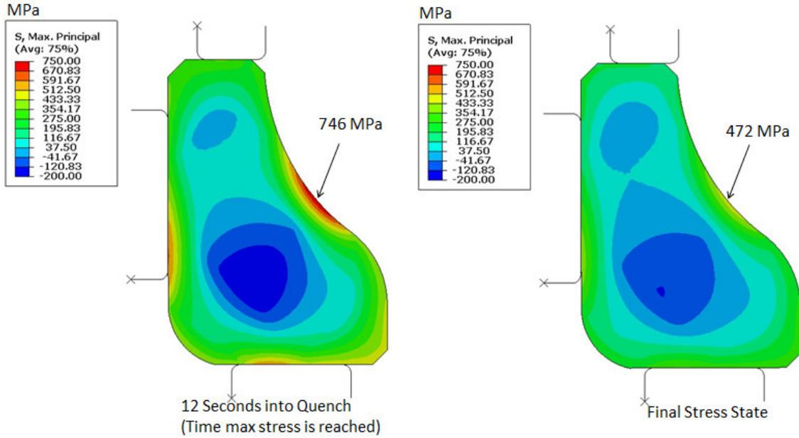
Figure 10 – Maximum principal stress at 12 seconds into press quench and at the end of the press quench, for the high heat transfer quench condition. (Case #5 in Table 2.)
