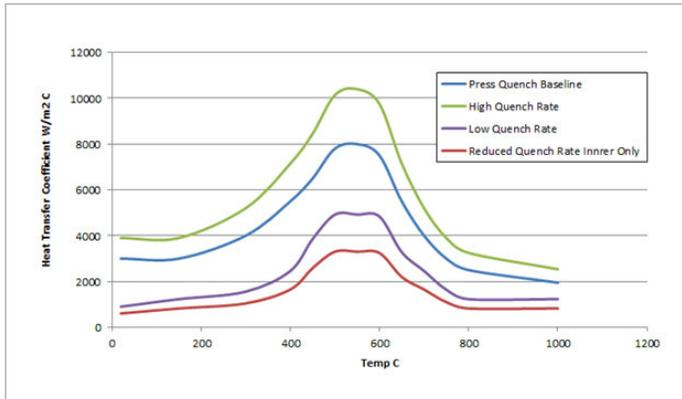
**Figure 5 – Heat transfer coefficient as a function of temperature for the four (4) quenching scenarios examined in this investigation.**
