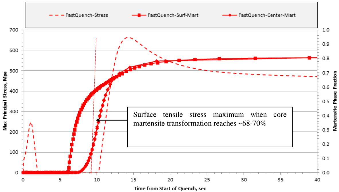
Figure 17 – Stress-Martensite-Time plot for the high heat transfer press quench (Case #5), showing how the delayed core transformation produces the transient tensile stress “spike” on the outer ring surface.
