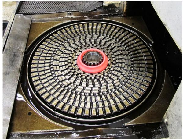
**Figure 3 – The hot inner bearing ring is shown positioned on the lower die assembly of a quenching machine just prior to quenching. Note the segmented lower die tooling and the individual slotted rings. These rings can be rotated independently to meter the flow of oil over the part being quenched.**
