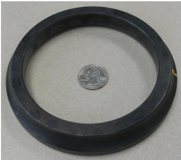
**Figure 1 – Inner bearing race.**
