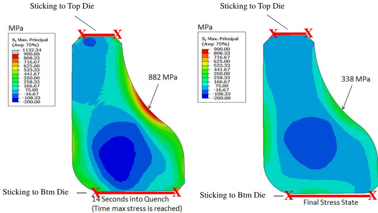
Figure 11 – Maximum principal stress at 14 seconds into press quench, with “Sticking” of both the top and bottom ring surfaces (radial displacement restriction). (Case#6 in Table IV)
