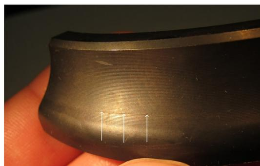
(a) Low Magnification of Crack.
