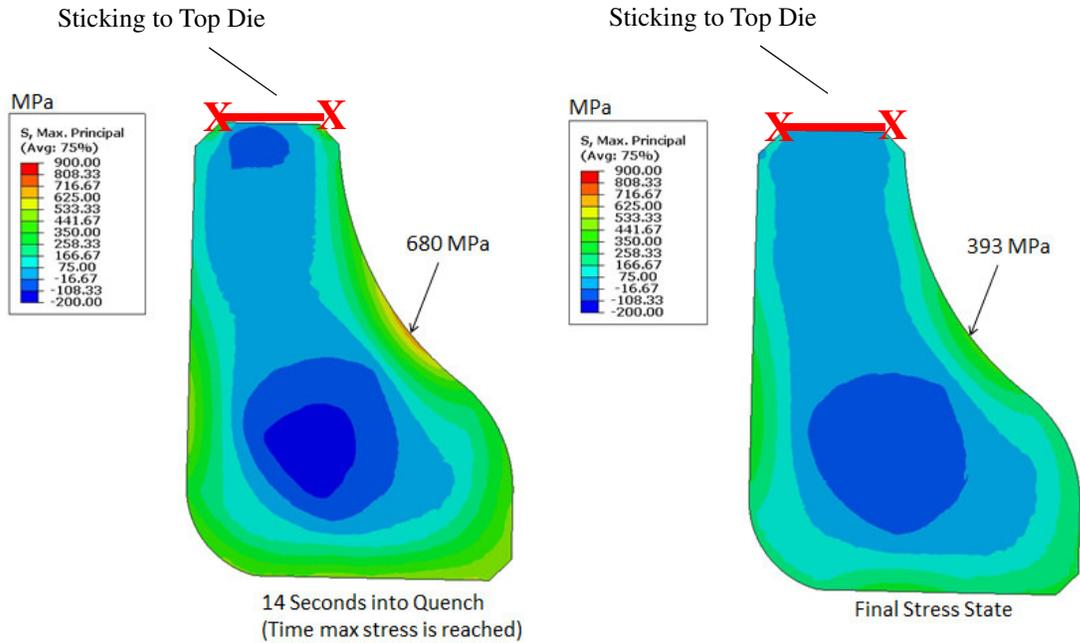
Figure 12 – Maximum principal stress at 14 seconds into press quench, with “Sticking” of the ring top surface (radial displacement restriction). (Case #7 in Table IV)
