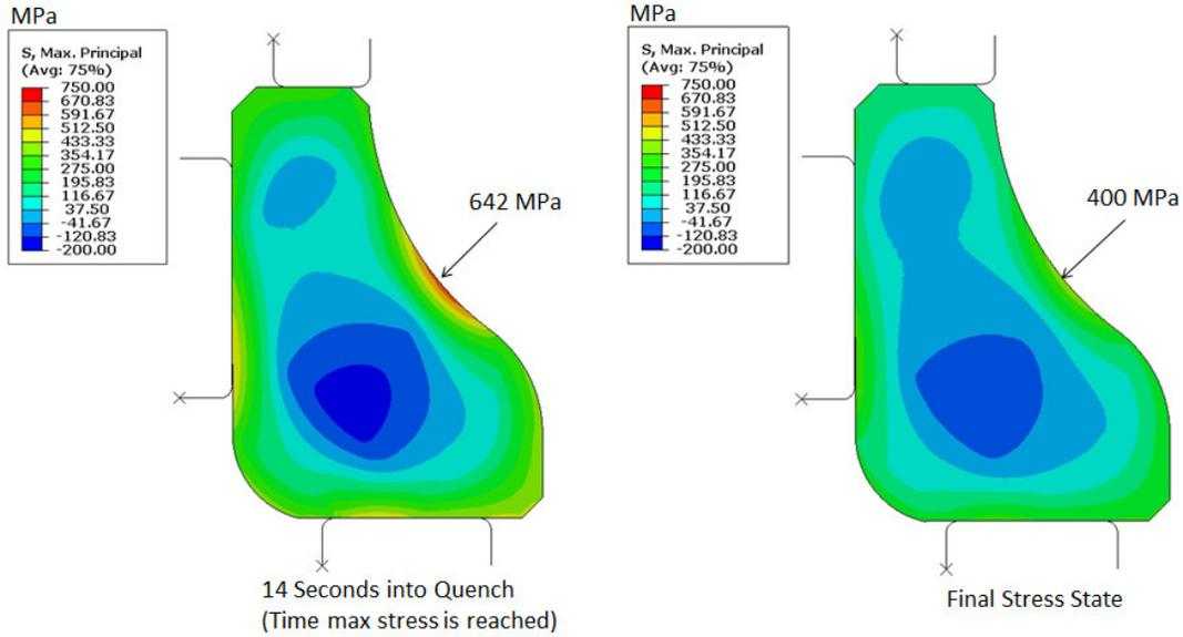
Figure 8 – Maximum principal stress at 14 seconds into press quench and at the end of the press quench for the baseline condition (Case #1 in Table IV)
