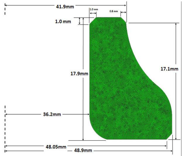
**Figure 2 – Cross-sectional profile of the asymmetrical inner bearing ring geometry that was studied during this investigation. The profile area was divided into 9,367 nodes and 9,188 elements for finite element modeling purposes.**
