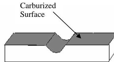
Figure 2. Schematic of Test Sample showing Carburized Surface
