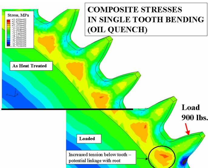
Figure 21. Cross Section Contour Map of Residual Stress in Oil Quenched Gear for Unloaded and Loaded Conditions
