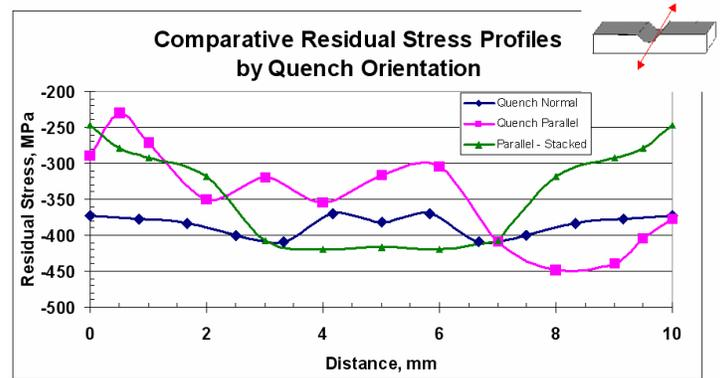
Figure 9. Comparison of Predicted Surface Residual Stress Across the Root of the Sample Notch.
