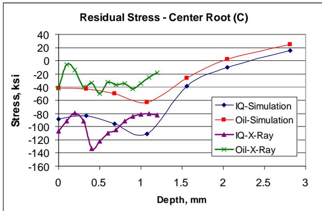
Figure 19. Residual Stress Profile Comparison at Position (C) in Test Gear for Simulation and X-Ray Calculations
