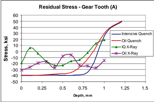
Figure 17. Residual Stress Profile Comparison at Position (A) in Test Gear for Simulation and X-Ray calculations
