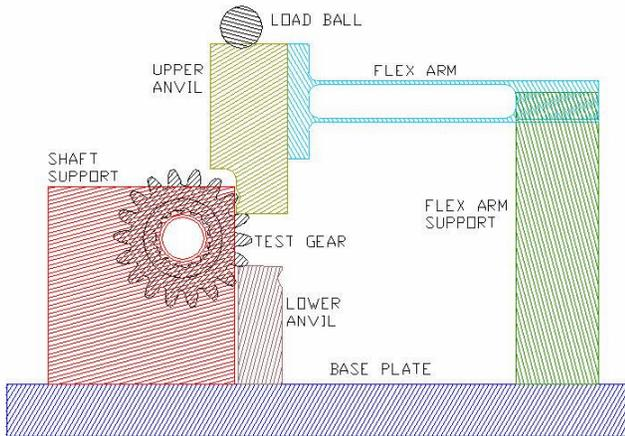
Figure 14. Schematic of Single Tooth Bending Fatigue Test Set-up
