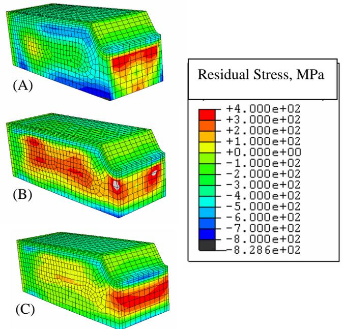
Figure 10. Predicted Cross Section Residual Stress Contours for 3 Quench Configurations
