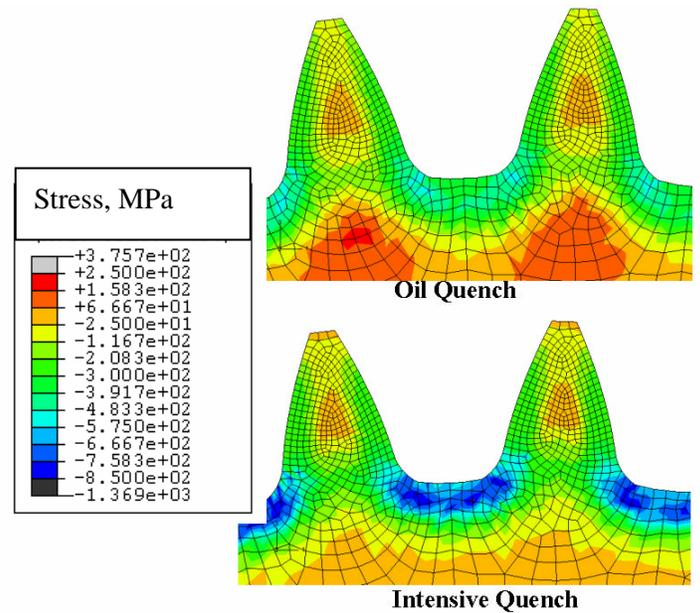
Figure 15. Residual Stress Profile Comparison after Heat Treat through Tooth/Root Cross Section
