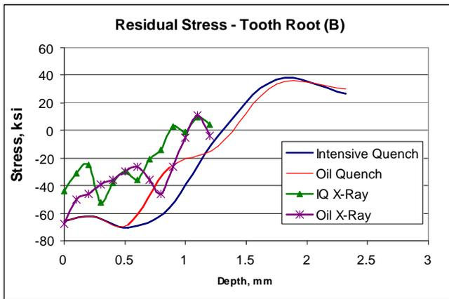
Figure 18. Residual Stress Profile Comparison at Position (B) in Test Gear for Simulation and X-Ray Calculations
