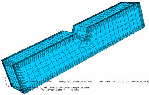
Figure 3. Finite Element Mesh of Test Sample
