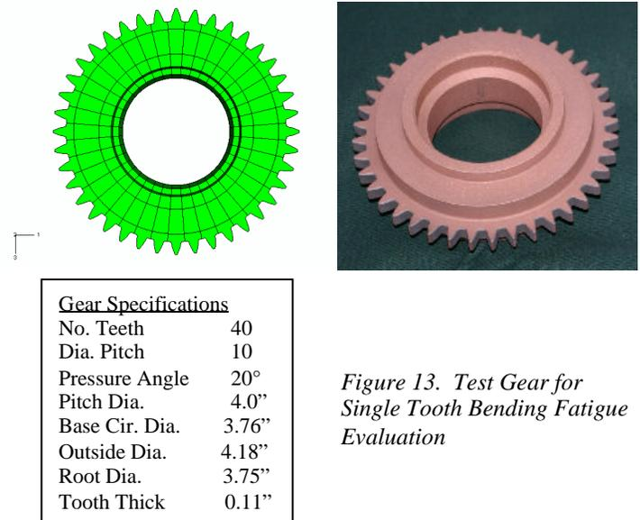
Figure 13. Test Gear for Single Tooth Bending Fatigue Evaluation
