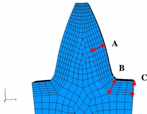
Figure 16. Reference Directions Points in Tooth/Root Cross Section
