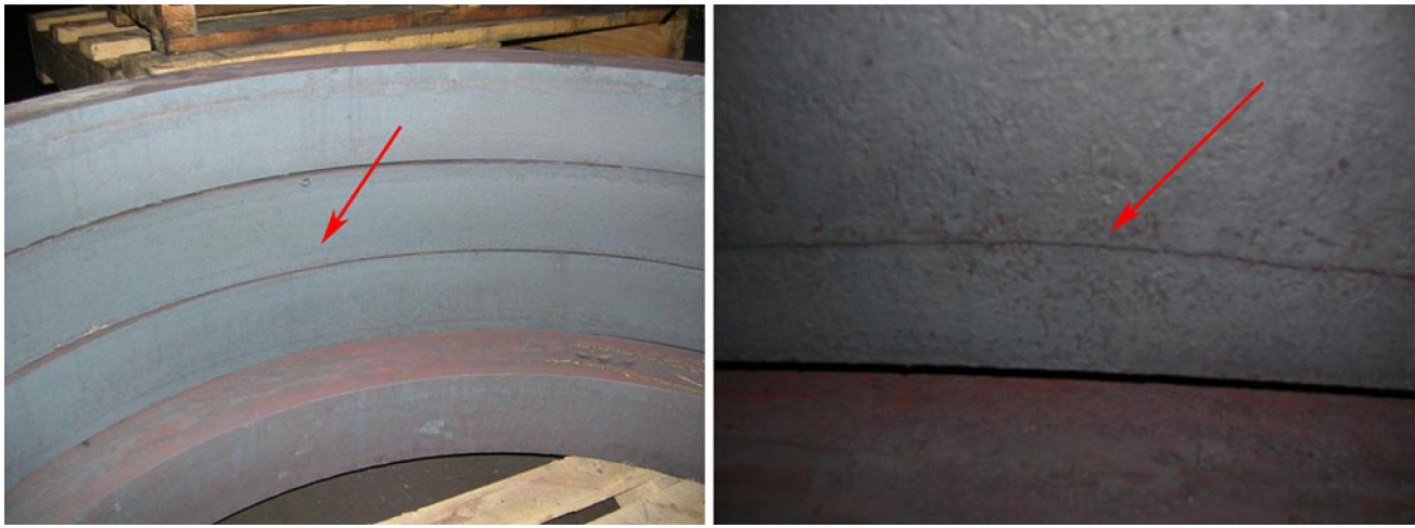
Fig. 1 Example of quench cracking of large rolled rings, with cracking emanating from the inner bore
