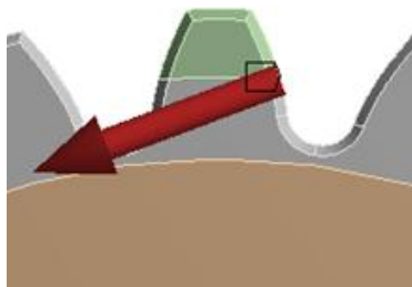
Figure 5. Static point load is applied normal to the surface at the pitch line.
