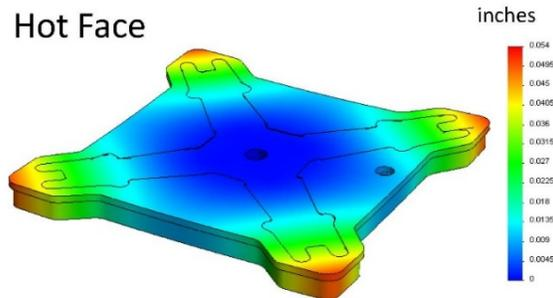
**Figure 2. Displacement measurements of the hot face of the mold insert after cooling to room temperature.**
