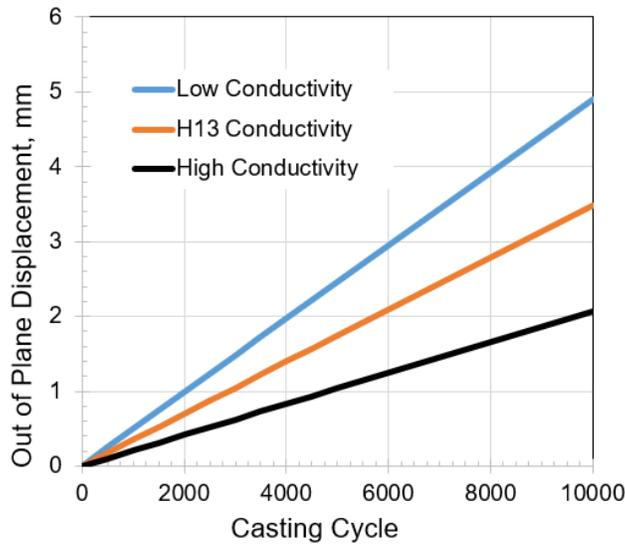
Figure 13. Extrapolation of model distortion prediction results to 10,000 casting cycles.
