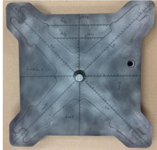
**Figure 1. Permanent mold insert showing lines used for measurements. The spacings are 0.25 in. (6.35 mm).**
