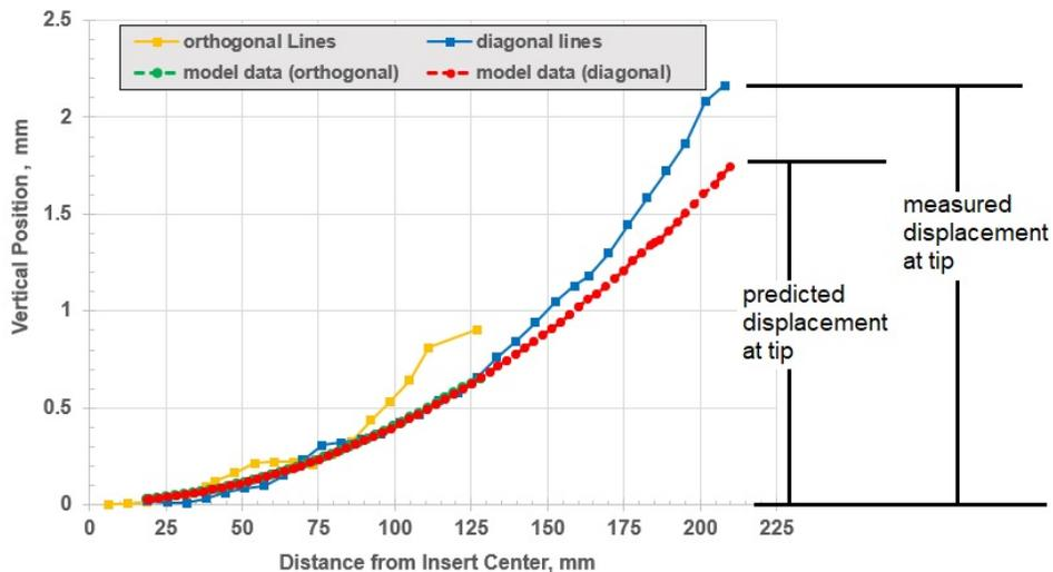
**Figure 12. Comparison of model predictions for 5,000 casting cycles and measurements for the distorted mold insert.**
