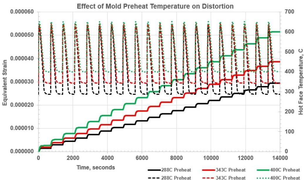
**Figure 10. Predicted strain and temperatures for the indicated mold preheat temperatures for twenty casting cycles.**
