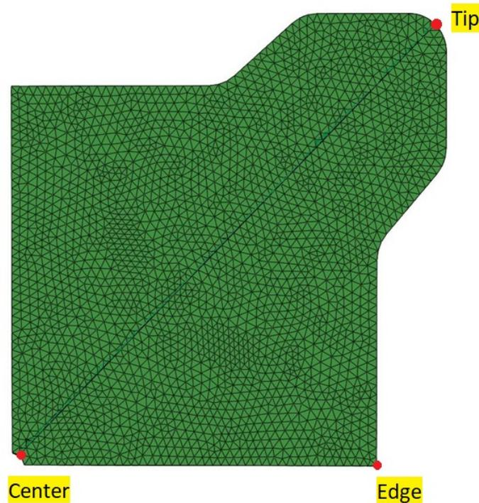
**Figure 7. Mesh defined to model the mold insert. A quarter view shows two one-eighth sections, each with 35,750 nodes and 86,809 tetrahedral elements and 36,708 wedge elements. Locations referenced in later figures are indicated.**
