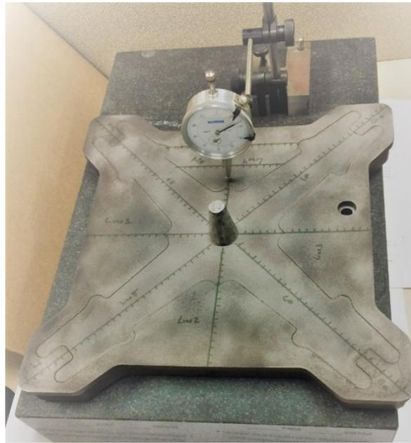
**Figure 3. Mold insert showing the measured lines and locations, dial indicator, and the granite block used for measuring flatness.**
