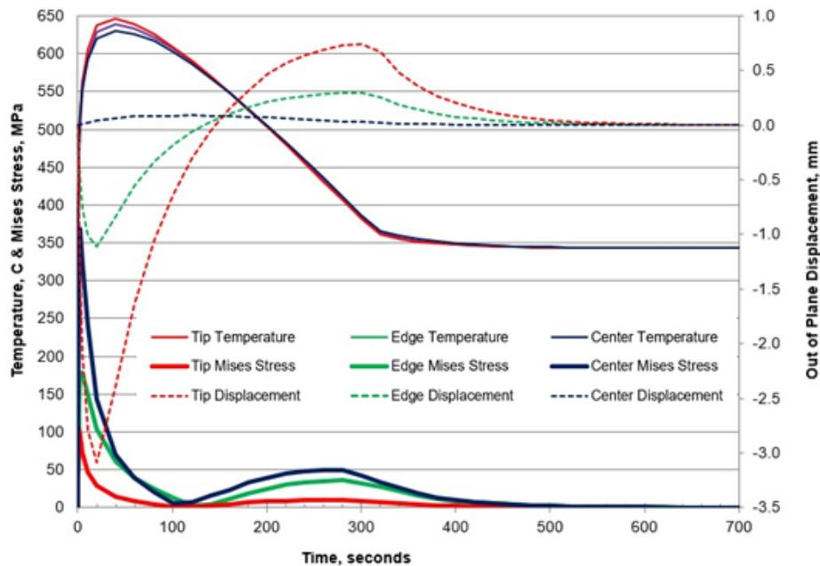
**Figure 8. Predicted temperature, von Mises or equivalent stress and out-of-plane displacement for three locations of the hot face during the first casting cycle. Tip is the mold insert outer corner, edge is the middle of a straight edge location, and center is the mold insert center location.**
