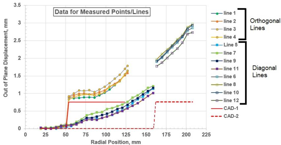
**Figure 4. Hot face measurement results for orthogonal and diagonal lines. CAD-1 and CAD-2 refer to original positions of the hot face planes, with the 0.030 in. (0.76 mm) recess evident in the line traces.**
