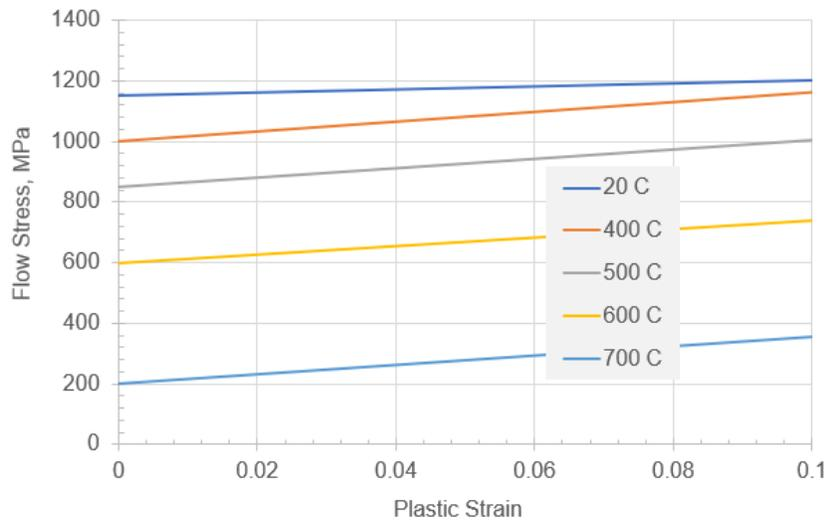
Figure 6. Flow stress properties used for model material.
