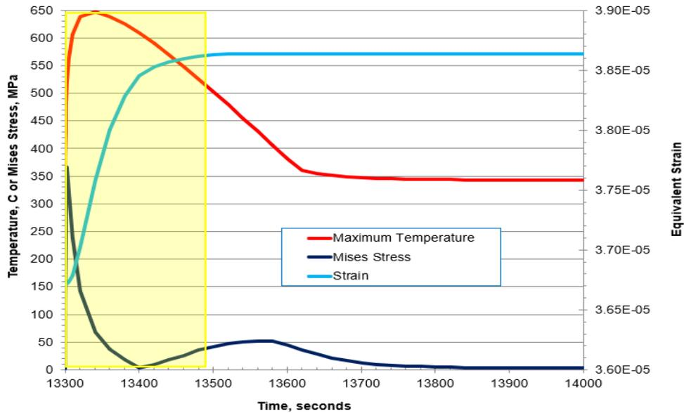
**Figure 9. Graph showing the temperature, equivalent strain and von Mises stress for the 20<sup>th</sup> casting cycle. The shaded box shows the temperature and stress conditions that result in permanent strain or distortion. The localized creep deformation accumulates with each casting cycle.**
