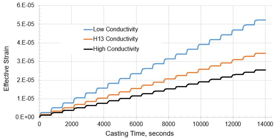
**Figure 11. With no change in hot strength and creep resistance, a mold material with higher thermal conductivity will distort less than a material with lower thermal conductivity. The plot is for strain build-up over twenty casting cycles.**
