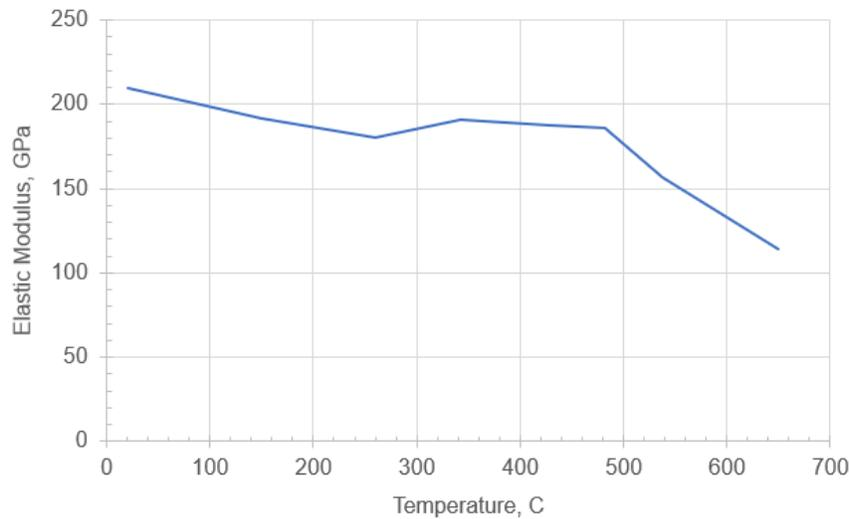
Figure 5. Elastic modulus used for model material.
