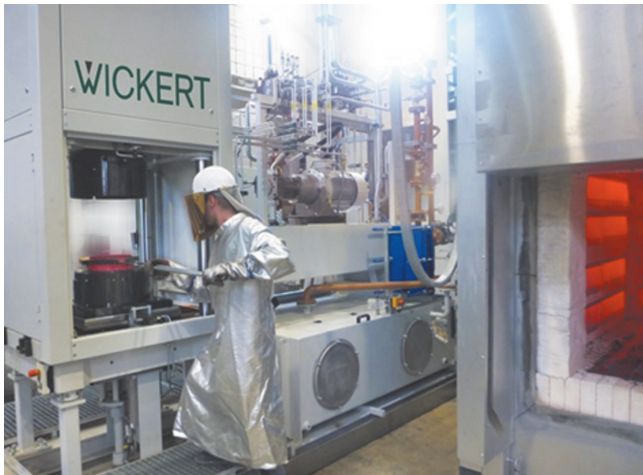
Fig. 5. Hardening press used for the experiments (Wickert Maschinenbau GmbH)
