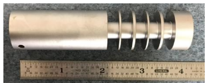
Figure 2. (a) LPC coupon drawing (unit: mm), and (b) Picture of fabricated coupon.
