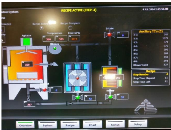
Figure 3: Human Machine Interface on DCGQ prototype unit showing process monitoring functionality.
