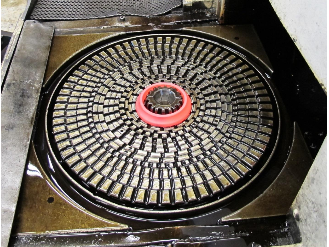
Figure 1. The hot inner bearing ring is shown positioned on the lower die assembly of a quenching machine just prior to quenching. This ring served as a part of the pulsing trials conducted during this investigation. Note the segmented lower die tooling and the individual slotted rings. These rings can be rotated independently to meter the flow of oil over the part being quenched.
