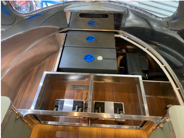
Services under bed area include water tanks, 2 x batteries, water/air heater and water pump
