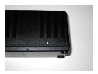
To adjust the speed, insert a small blade type screwdriver through the case to engage the potentiometer. Speed is increased by turning clockwise. Use a strobe disc and a fluorescent light source to aid in your speed adjustments. Note that the speed is set ever so <u>slightly</u> on the fast side at the factory to compensate for stylus drag.
