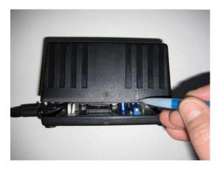
While lining up the base with the top of the case, make a mark with a pencil in line with the center of the blue adjustment pot as shown. Then mark a horizontal line exactly 6mm up from the bottom edge of the cover to intersect the first line. This marks the spot to drill a 9/64" hole.
