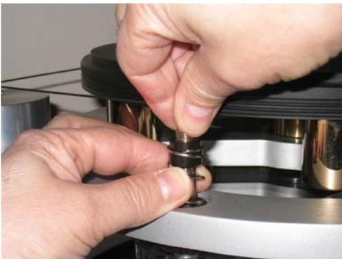
18. Install the three spring covers making sure they seat fully on the chassis.
