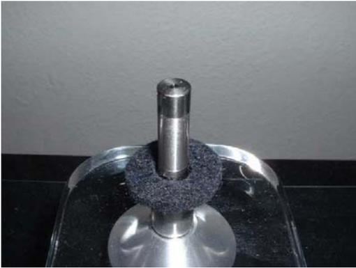
3. Screw the spring assemblies onto the threaded spring support sleeves until all the threads are fully showing above the black Delrin bushing. Then locate the three hollow spring support towers onto the three support spindles on top of the acrylic spider. Drop the white Teflon rings on top of each spring base. **NOTE: When handling the support towers, make sure not to lose the thrust ball that sits inside the sleeve of each tower.**
