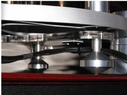
14. Now carefully lower the platter over the threaded record spindle and secure it in place with the knurled platter nut, insuring that the nut's recessed side is facing downward. Connect the power supply lead to the motor lead.
