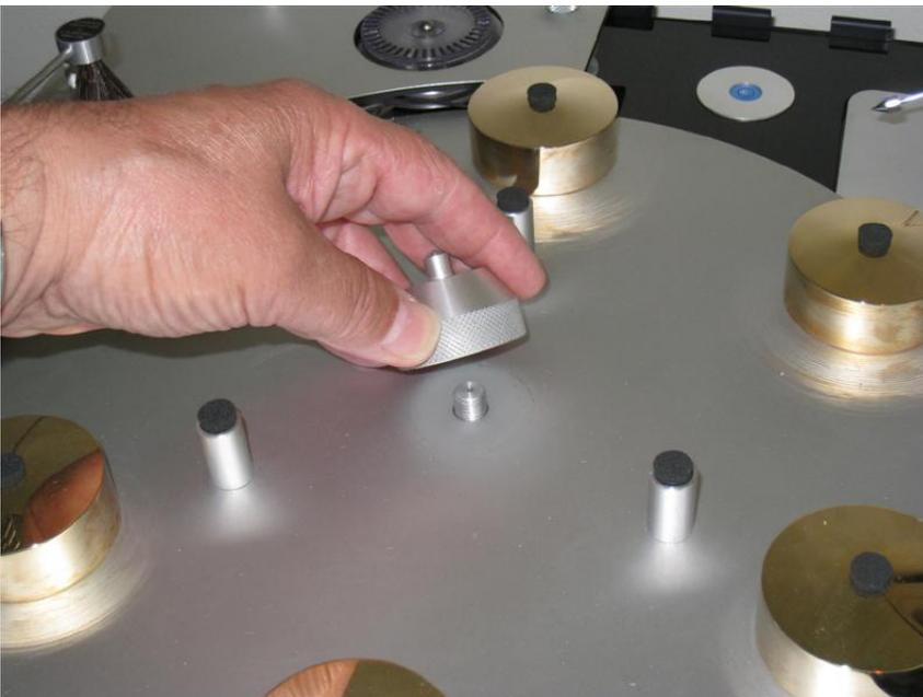
Use your thumb to push down on the centre spindle while lifting the platter. **Make sure the centre spindle stays fully seated in the bearing as you lift the platter off.** This will insure that the red interface washer that couples the fluid well to the bearing shaft is not torn or damaged.
