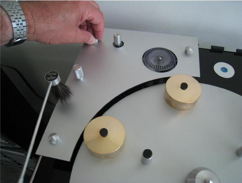
Undo the knurled platter hold-down nut
