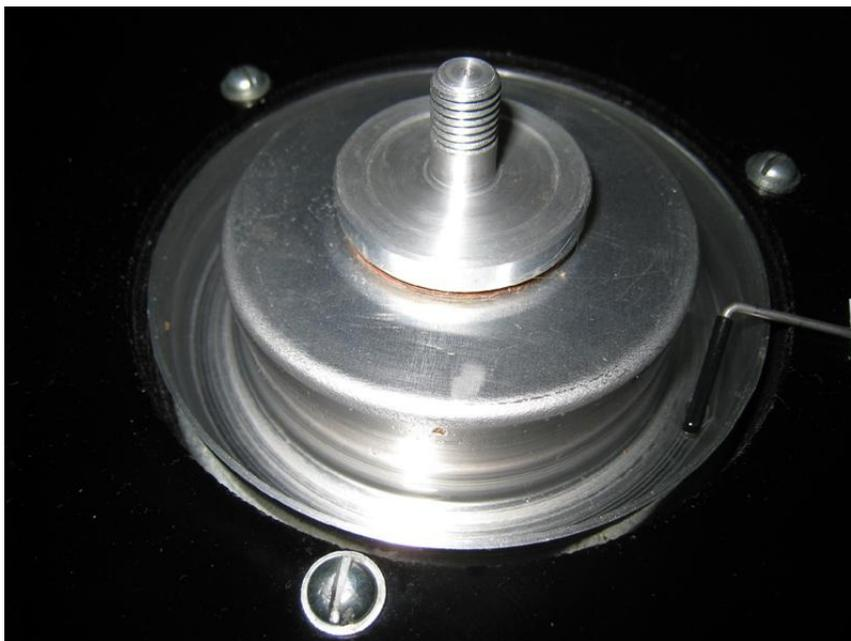
Reinstall the platter without the belt and give it the slightest push with one finger to get it rotating. It should spin friction free for a few revolutions. If it does not, you are most likely missing the thrust ball. Reinstall the belt and motor top plate. This is how the belt should look.
