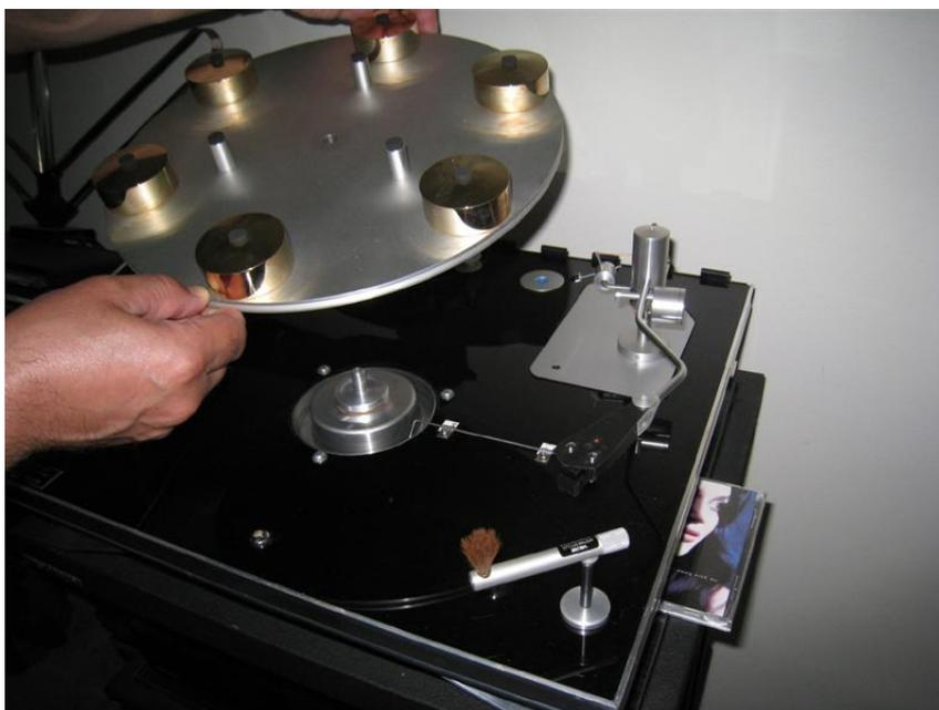
Undo the two Philips head screws that secure the speed control wand to the deck. This photo also shows what a main bearing with an undamaged interface washer looks like. The well will be connected to the spindle and spin together as a unit.
