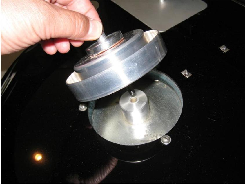
Re-install the speed control wand. Do not over tighten the screws or you will strip the wood. You should feel some snugness when you push the silver control knob back and forth so it will stay where it is put. Otherwise the fluid will move the speed control, changing the set speed.
