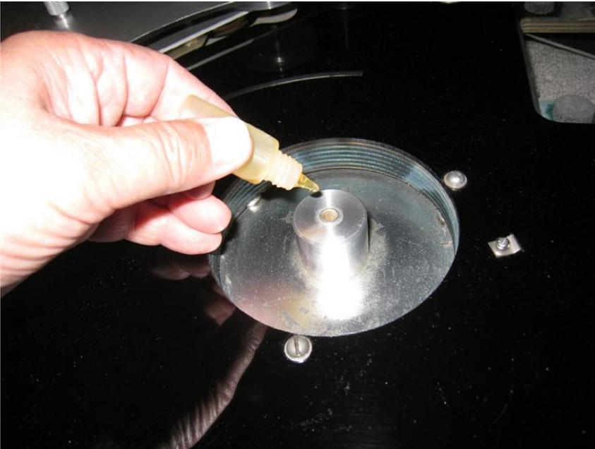
Replace the bearing assembly. Spin it by hand to make sure it spins freely. Also verify that the fluid well does not exhibit excessive vertical or horizontal run out. This would indicate that the fluid well is bent. It can be carefully bent into correct position if necessary, but be careful not to break the glue joint. It does not have to be perfect but is better if it is.
