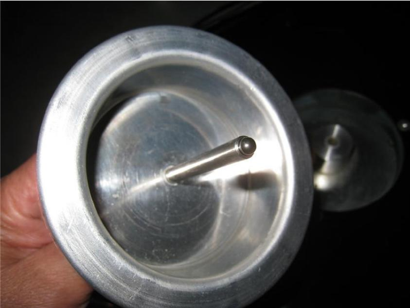
If the ball is not on the end of the bearing shaft verify that it is in the bottom of the bearing hole using a flashlight.
