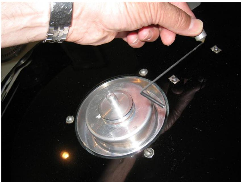
Remove the main bearing shaft and fluid well assembly. Be careful not spill any silicone fluid or to lose the round thrust ball bearing. It sits in the bottom of the bearing hole but sometimes sticks to the bottom of the bearing shaft.
