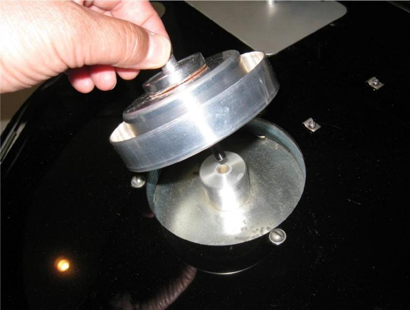
This is what the thrust ball looks like if it comes out with the bearing shaft. Set the ball aside so you don't lose it.
