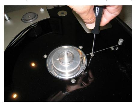
If necessary you can add paper shims to tighten up the wand. Paper from a credit card works well for this.
