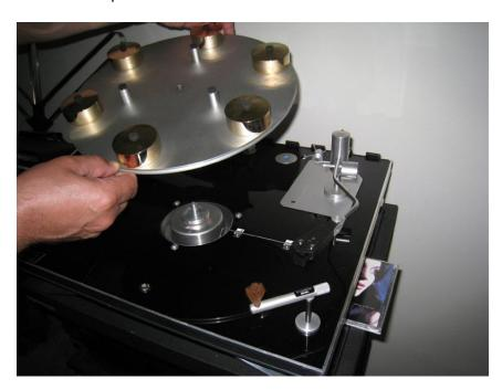
Undo the two Philips head screws that secure the speed control wand to the deck. This photo also shows what a main bearing with an undamaged interface washer looks like. The well will be connected to the spindle and spin together as a unit.
