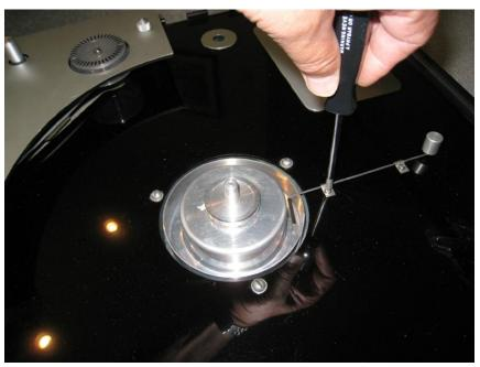
Lift off the speed control wand. Wipe any silicone fluid off the black paddle and set aside.
