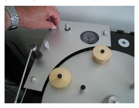
Undo the knurled platter hold-down nut
