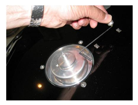
Remove the main bearing shaft and fluid well assembly. Be careful not spill any silicone fluid or to lose the round thrust ball bearing. It sits in the bottom of the bearing hole but sometimes sticks to the bottom of the bearing shaft.
