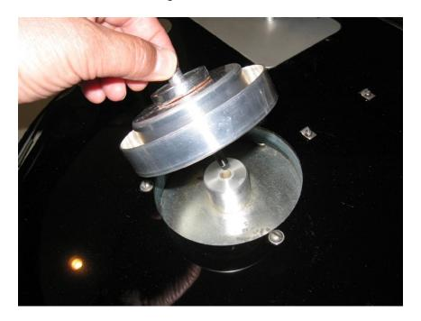
This is what the thrust ball looks like if it comes out with the bearing shaft. Set the ball aside so you don't lose it.
