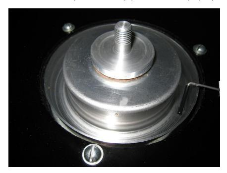
Reinstall the platter without the belt and give it the slightest push with one finger to get it rotating. It should spin friction free for a few revolutions. If it does not, you are most likely missing the thrust ball. Reinstall the belt and motor top plate. This is how the belt should look.
