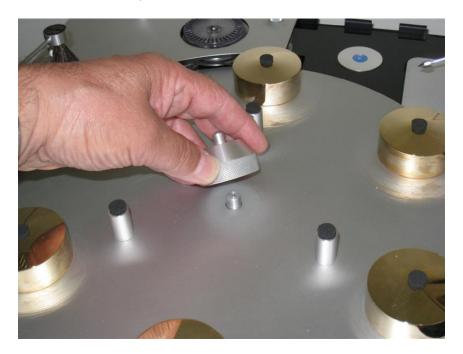
Use your thumb to push down on the centre spindle while lifting the platter. **Make sure the centre spindle stays fully seated in the bearing as you lift the platter off.** This will insure that the red interface washer that couples the fluid well to the bearing shaft is not torn or damaged.
