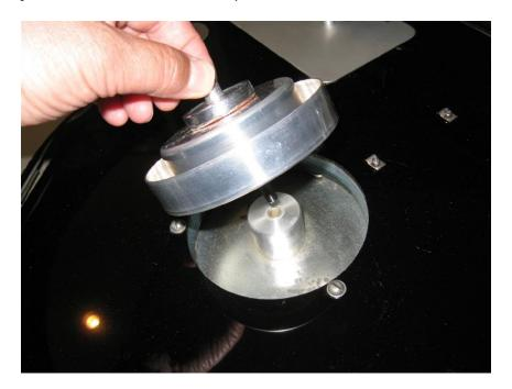
Re-install the speed control wand. Do not over tighten the screws or you will strip the wood. You should feel some snugness when you push the silver control knob back and forth so it will stay where it is put. Otherwise the fluid will move the speed control, changing the set speed.
