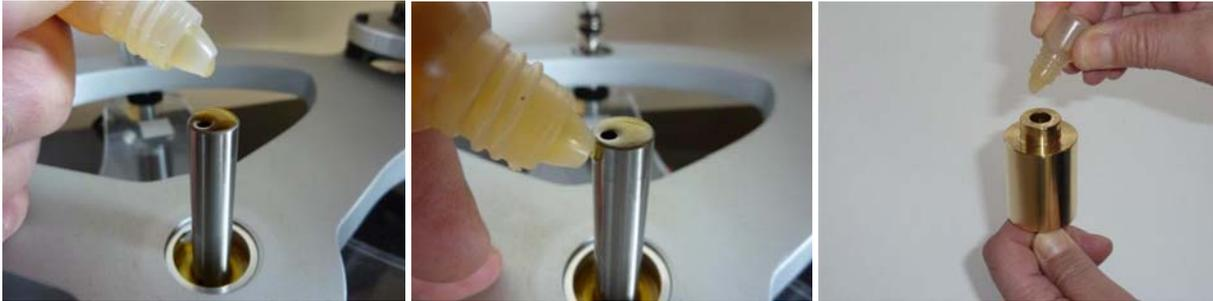
8. Making sure you do not lose the thrust ball, carefully lower the bronze housing onto the bearing shaft while gently rotating it back and forth to spread oil on all the bearing surfaces. Once fully home, spin the bearing six or more times with your thumb and forefinger to pump oil up into the top of the bearing. (The bearing pumps oil if spun clockwise only).
