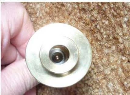
5. Squirt some lighter fluid into the bronze housing, cover the hole with your thumb and shake the housing to wash any oil from inside. Dump the contents onto a cloth or paper towel being careful not to lose the thrust ball if it was present. Repeat the wash cycle and set the bronze housing and thrust ball aside to dry.
