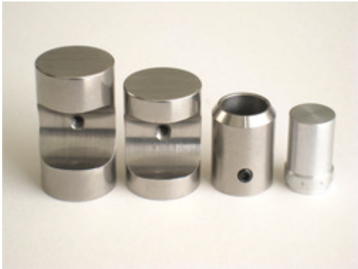
Left to right: Large weight, small weight, slider bush, finger adjuster.
