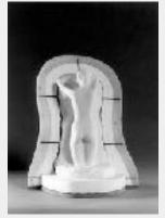
The surface of this second clay model is slightly scraped away. When this second model is returned to the mold, there is a gap between the model and the mold. This gap is where the wax will be poured. The final bronze will be of the same thickness as the gap that is created by the scraping.
