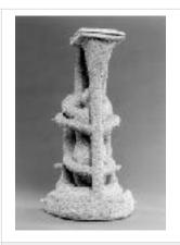
A finely granulated ceramic is applied to the surface of the model and its pipes until it becomes thick and coarse. The result, now called an "investment mold," is then dried and heated. This causes the wax to melt and flow out of the mold, leaving a space between the fire resistant clay model and the investment mold. This is why this method is called the *lost wax* process.
