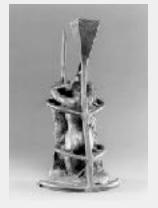
Except for a place to pour in the liquid bronze at the top, the mold is covered with a layer of cladding (a protective metal coating), which must be completely dry before bronze pouring begins. The investment mold is then heated to a high temperature (over 1,000 degrees Fahrenheit).
