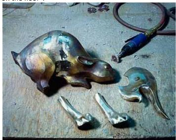
Any gates and vents are removed from each section of the sculpture and the pieces are then welded back together. One can realize the tremendous time and labor involved just up to this point.
