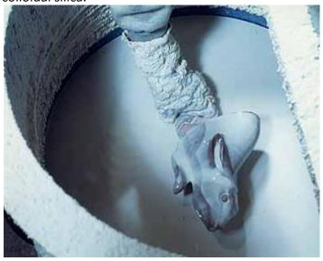
While it is still wet, the tree is coated with the first layer of sand which is made up of fused silica. This process takes about 8 days to complete. Each day it is dipped in slurry and once again coated with the silica sand. The silica sand used goes from very coarse to very fine beginning to end. Eventually the shell will be approximately 1/2 inch thick.
