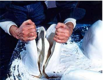
The next step is to remove the artists' original and reassemble the clean, empty mold. Now a way pattern will be poured by building several layers of the hot wax within the rubber mold. A layer is poured, allowed to dry until there is about a 1/4 inch thick wax pattern made of the artists' original. It is very important to note that the wax pattern is a hollow duplicate of the artists' original.
