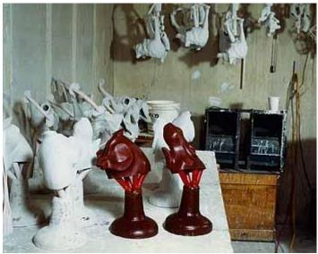
First the wax tree is dipped into a slurry tub and coated. The slurry itself is basically made up of colloidal silica.
