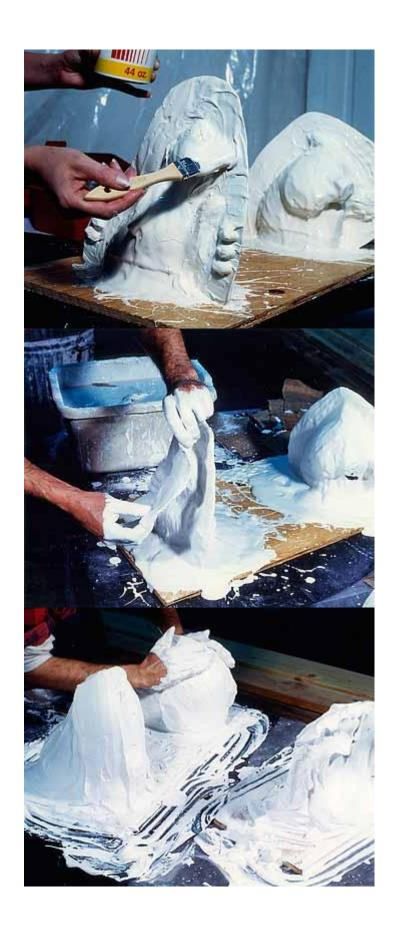
The "mother" mold is now complete, the next step is to separate the two halves of the mold and remove the original from inside.
