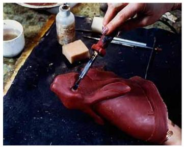
Eventually there will need to be a way for the hot, molten bronze to funnel its way into a ceramic type mold, shown here the wax pattern is sprued and mounted on a wax cup. The red spures serve as gates and vents later in the process.
