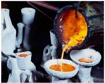
After the bronze is cooled, the shell cracks on its own accord and is manually removed from the bronze. This could also be called the "lost shell" method if casting. The sculpture is now "metal on the floor".
