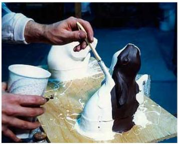
A lock and tab system has been applied (see the edge) so that the mold will be able to be opened and closed securely. Once the rubber mold has been completed, a plaster or fiberglass "mother" mold is applied to the outside which will preserve the integrity of the rubber mold.
