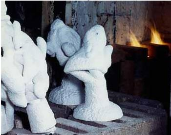
Now the shell is ready to receive the molten bronze. It is poured at a temperature of about 2,000 \*F.
