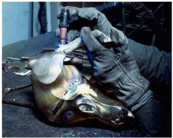
Once the pieces of the sculpture have been reunited, or welded back together, the weld lines are then tooled out and any imperfections in the metal are corrected. This takes place in the metal room where the critical talent of the artisan's transforms the parts into a hollow bronze duplicate of the original clay model.
