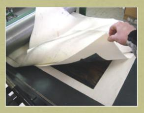
from the incised marks and not from the top surface of the plate, although thin films of ink may be left on the surface to produce a variety of tonal effects. For intaglio printing, the paper is dampened so that under printing pressure it will be squeezed into all the inked recesses of the plate and around it (leaving a PLATE MARK if the plate is smaller than the paper).
