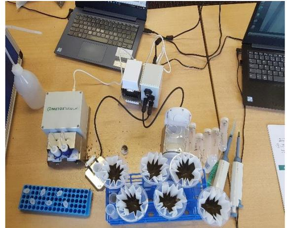
Figure 1: MobiLab testing for nitrogen levels within freshly taken soil samples with a turnaround of 30 mins.
