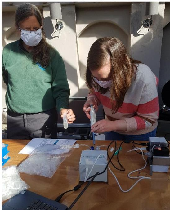
Figure 2: WRT staff get to grips with the Mobilab, testing for Nitrogen levels within plant tissue, water & soil samples.
