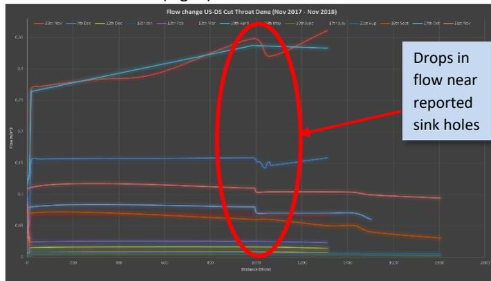
Figure 7: Flow losses within the CTD
