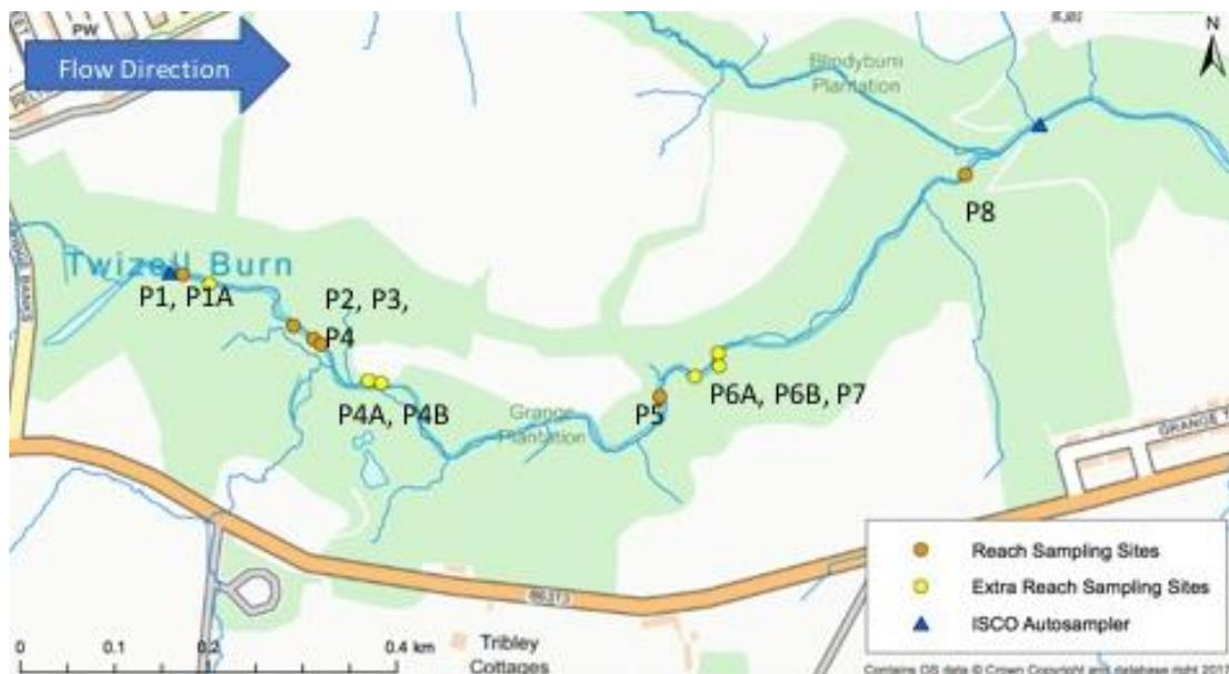
Figure 1-4: Reach sampling locations, showing the sites of piezometers and ISCO-3700 auto-samplers.
