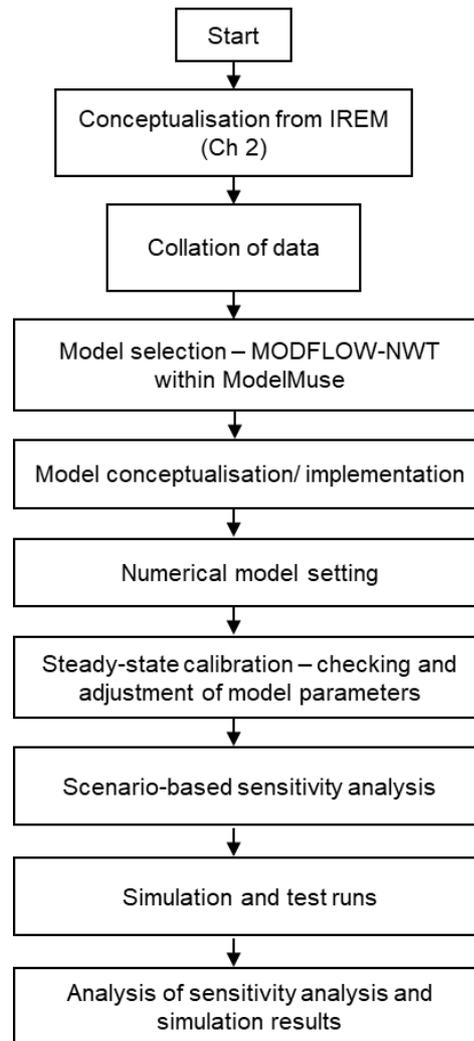
*Figure 1-7: Steps taken to develop a numerical model representing the Twizell Burn reach using MODFLOW-NWT.*
