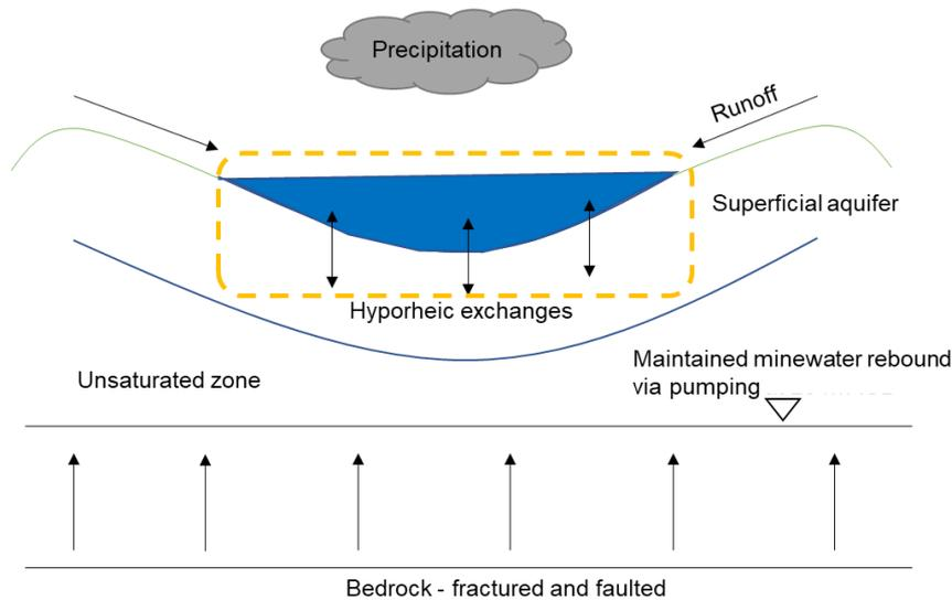
Figure 1-6: Conceptual cross-section of the Twizell Burn GW/SW systems, highlighting direct inputs into the systems and the shallow hyporheic exchanges within the minor aquifer.
