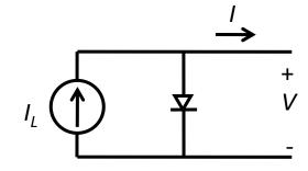
Note: this reduces to a simple Diode in the dark  $(I_L = 0)$
