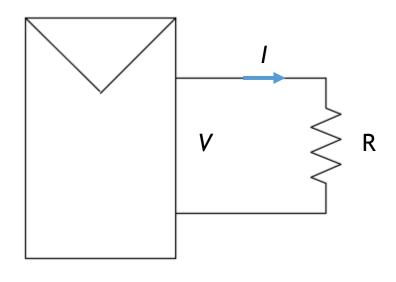
Operating point for a given resistance is found by the intersection of the IV curve with the line whose slope is 1/R
