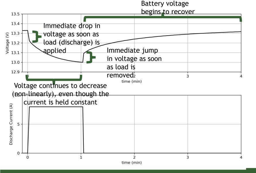
Battery voltage before and after a load of 8A is drawn from the battery (12V, 100 Ah, AGM Battery)
