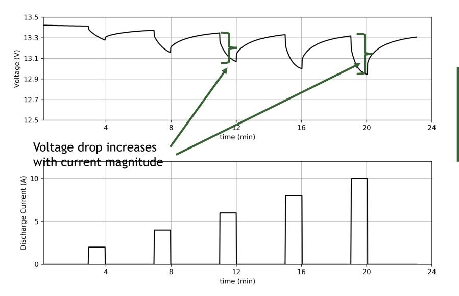
Battery voltage as succession of larger discharge current with 1 minute rest in between is applied (12V, 100 Ah, AGM Battery ~75% SoC)
