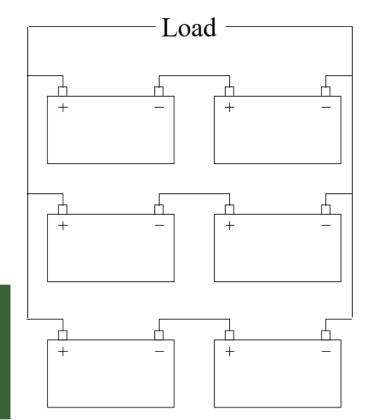
Consider the battery bank shown consisting of six 12V, Renology AGM 200 batteries. Compute the battery bank voltage, charge capacity, and energy capacity at the 20 hour rate.
