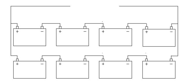
In other words, the battery bank is equivalent to a single 24 V, 750 Ah battery
