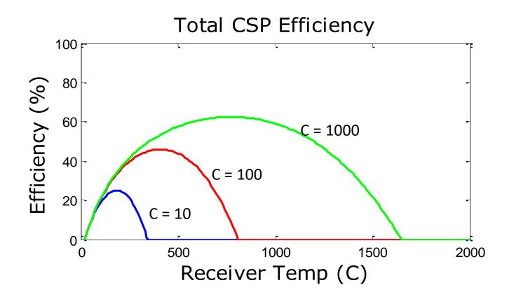
A typical concentration ratio for a PTC CSP is 70. Find the receiver efficiency, Carnot efficiency and total efficiency if:
