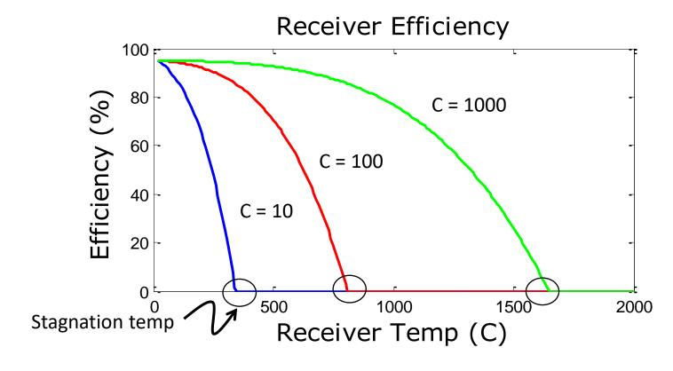
With:  $T_{amb}$  = 20 C;  $\varepsilon$  =  $\alpha$  = .95;  $G_{DNI}$  =770 W/m<sup>2</sup>
