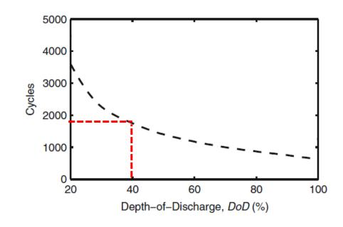
lower than 40%, so battery will last longer than 1825 cycles
