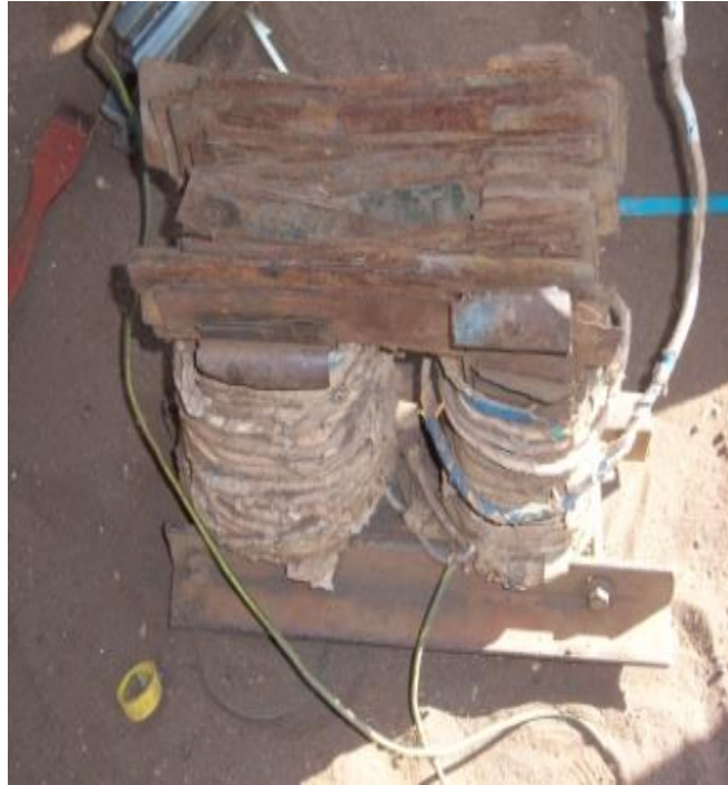
“homemade” Zambian transformer
