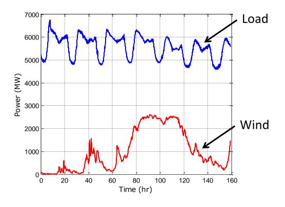
Note: Total Wind Plant Capacity is 2780 MW
