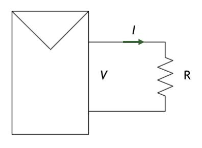
Operating point for a given resistance is found by the intersection of the IV curve with the line whose slope is 1/R
