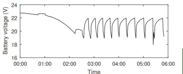
Inverter reconnects and quickly disconnects. (this is early in the morning when there is no PV power)
