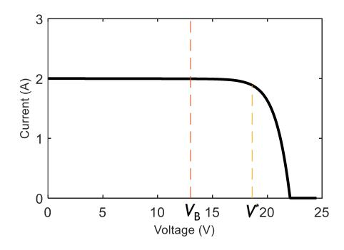
Next, consider the scenario in which the house has an MPPT (boost converter) that is connected between the module and the battery. The voltage and current corresponding to the maximum power point are 18.7 V and 1.89 A. Compute the duty cycle so that the PV module operates at its maximum power point and the corresponding power and current into the battery.
