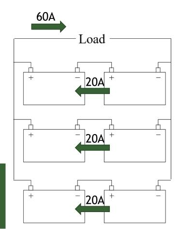
• Estimate how long the battery bank can supply a 60 A load until the cut-off voltage is reached?
