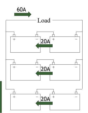
• What is the energy capacity when the battery bank is discharged at 60A?
