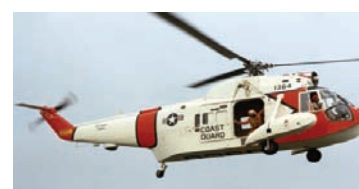
Sikorsky HH-52A Seaguard was an amphibious single turbine engine helicopter attached to Air Station Salem and later moved to Cape Cod. This helicopter made rotary-wing aviation the backbone of Coast Guard search and rescue.
