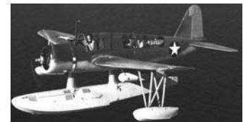
Vought OS2U Kingfisher had the flight capability of 6 hours per mission. Photo: cgaviationhistory.org
