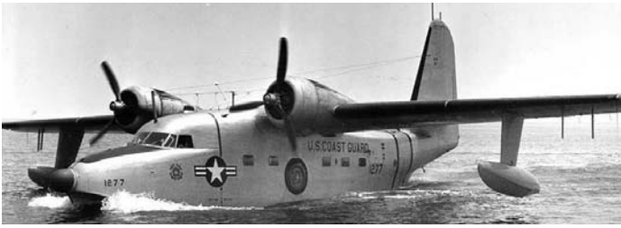
Albatross UF-1G Grumman Model G-64 (later known as the HU-16E) was the largest of a series of amphibians designed and manufactured by the Grumman Aircraft Corporation for the military. It was stationed at Air Station Salem beginning in 1951. Photo: US Coast Guard Aviation History project
