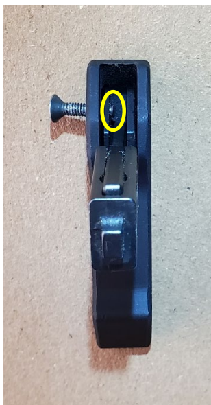
Place FCH on the side as shown. Note: Keep screw tip flush with base interior wall (photo shows screw tip incorrectly extended beyond interior wall)
