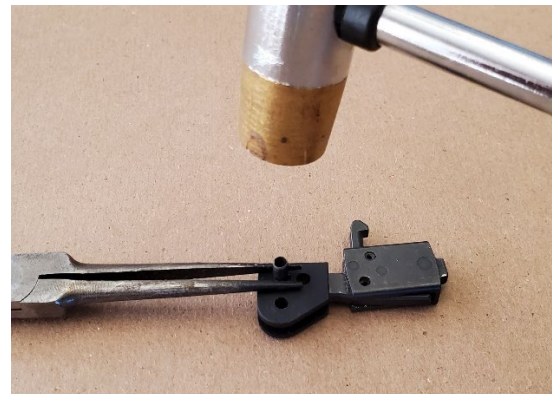
Slide the base over the carrier arm, Pinch the slotted pin with the needle nose pliers, place the pin over the upper hole as shown and tap in ever so slightly to where the pin is captured. Align the pin holes with the carrier arm holes and drive the pin all the way in. Note: Notice base orientation and carrier hook.
