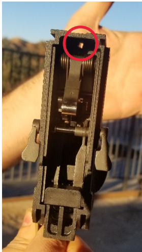
10. 1/8" hole daylight through firing group cavity.
