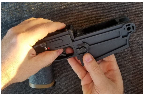
3. Slide the mag-well half of the receiver off and set aside.
