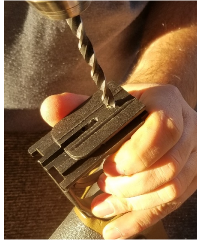
11. Using the 1/4" drill bit, drill the receiver's upper hole. Apply light pressure while drilling to avoid the drill bit slamming into the hammer.
