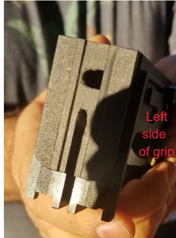
12. Using the 1/8" drill bit, drill 2 additional holes to the RIGHT side of the 1/4" hole and square the hole in a reversed "D" shape as shown. This step can also be done with the utility knife. Next step is to insert the link.
