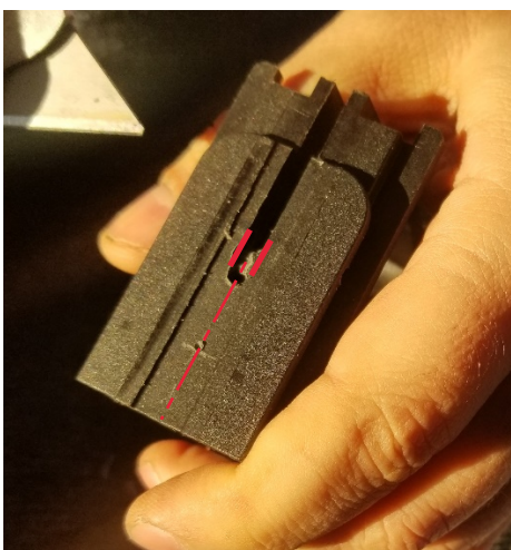
10. Using a utility knife, cut the receiver slowly along the existing channel side walls to extend the channel to the new 1/8" diameter hole.
