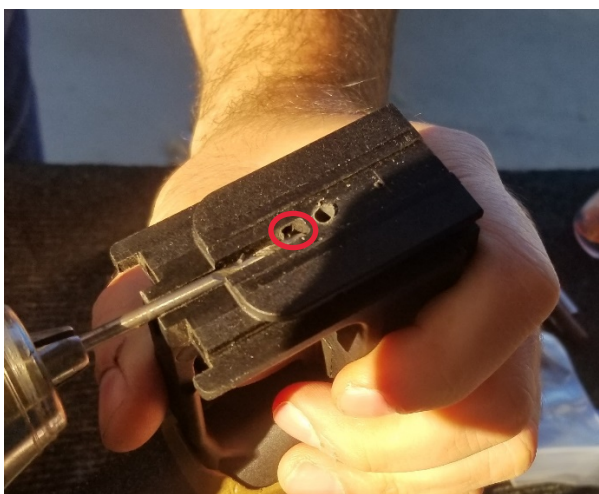
9. Using the 1/8" drill bit, drill the lower receiver sideways inside the channel, through the end wall, until the bit comes out inside the firing group cavity.
