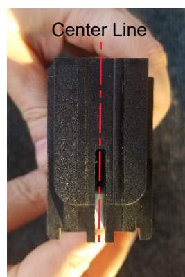
4. Drilling will be on this face of the lower receiver.
