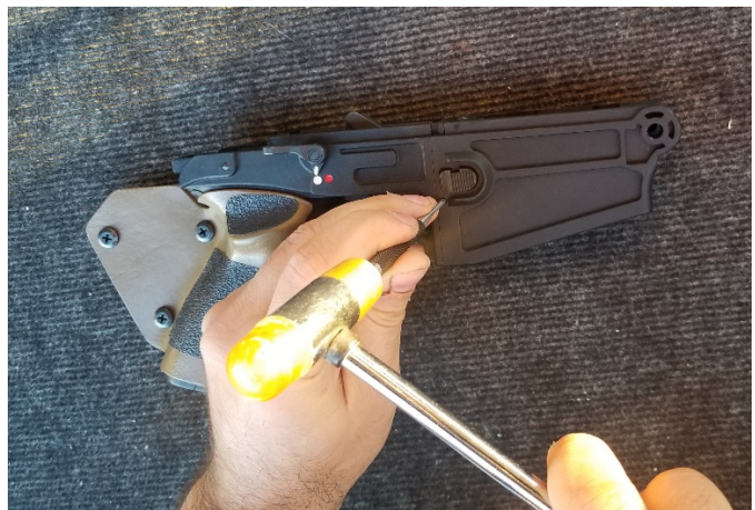
2. Using a punch tool, remove the roll pin out.
