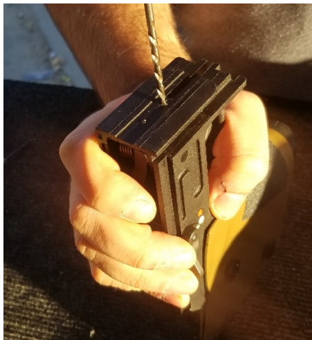
8. Using the 1/8" drill bit, drill the receiver's lower hole. Hole must be no deeper than 1/4".
