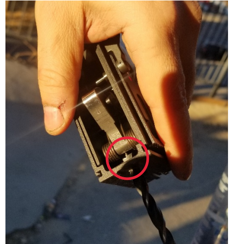
11. Using the 1/4" drill bit, drill the receiver's upper hole. Apply light pressure while drilling to avoid the drill bit slamming into the hammer.
