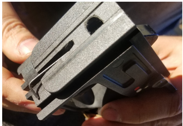
13. insert the link into the receiver by lowering it down the firing group cavity and out the 1/8" hole with the tail pointing outwards. Once the link nose is inside the firing group cavity, rotate the link 180 degrees where the nose is pointing outward and the tail will be pointing towards the trigger guard .
