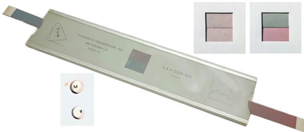
Figure 1 The D & H Color Rule. Look closely to see the wildly different reflectance curves representing the colorants used on the two sliders. The upper right images show one match as seen under two different light sources (or by two different observers). The bottom left image shows the settings from the back of the rule indicating the sliders' positions (M9) for a match.
