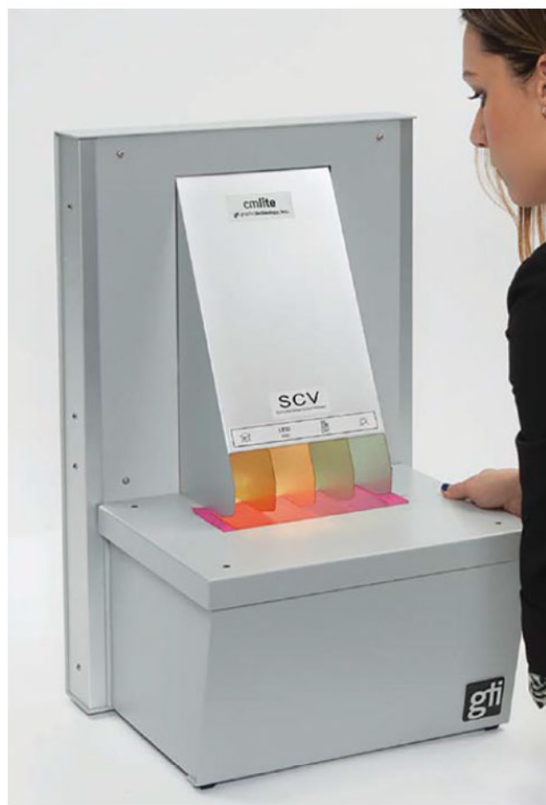
Figure 2 The GTI Simultaneous Color Viewer shows the impact of different lights on the color rendition of a single sample.
