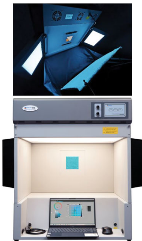
Figure 11. The LEDSimulator system. Top: Back view showing LEDPanels and a colored fabric swatch. Bottom view: Viewing area with 1) the aperture showing the chromaluculent colored fabric and a chromaluculent colored fabric swatch and 2) a laptop with ColorWay software.
