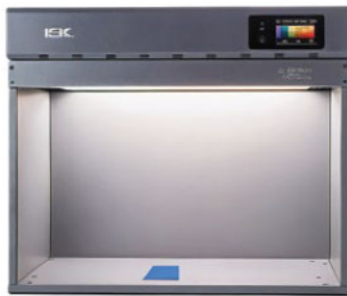
Figure 3. Blue swatch illuminated by white light in a viewing cabinet. Illustration generated by newarc.ai.
