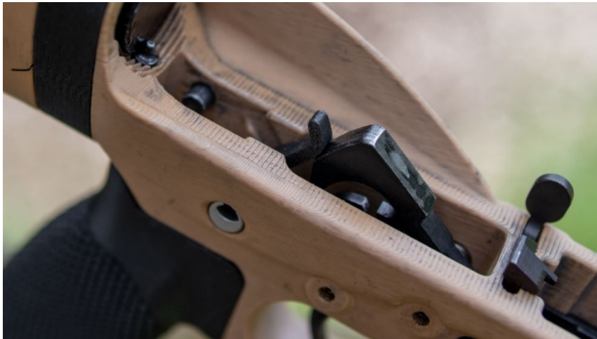
Figure 16. Super Safety installed in a lower.
