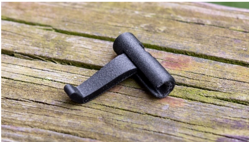
Figure 15. Test fitting the lever in the cam.
