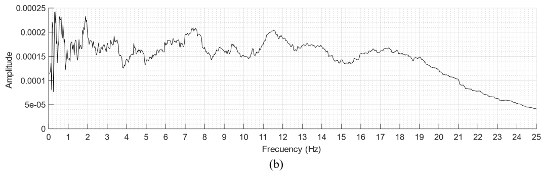
Figure 20. White noise: (a) signal and (b) Fourier spectrum.
