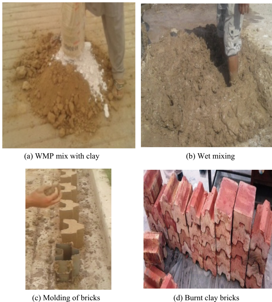
Fig. 4. Manufacturing process of interlocking bricks.
