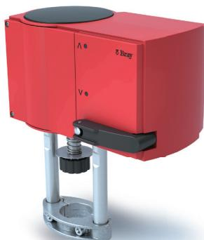
These actuators operate on 24V AC or DC, and all input signals- 0-10V or 4-20mA modulating output, or on/off (2-point) or floating (3-point) control, direct or reverse acting. The actuator automatically detects the control signal applied via a 2 LED display.
