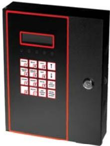
The M-Controller is a multi-channel controller and alarm unit. It utilizes both digital and analog communications to interface with a maximum of 32 remote digital transmitter/sensors, and 8 analog transmitter/sensors. Range and alarm setpoints are set either through the front keypad or through software that is downloaded to the controller from a PC or laptop computer. An additional feature includes 24 VDC transistor outputs for a horn and strobe.
