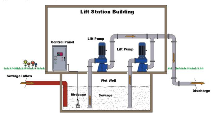
The purpose of the level transmitter is to provide feedback to the pump allowing them to turn on and off when the level reaches a set height. Floats, bubbler systems, radar and ultrasonic are all ways to indicate level. However these methods can have installation difficulties, maintenance issues, high costs or reliability issues due to the environment.
